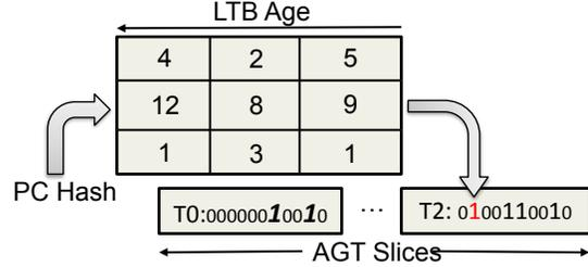
Figure 3: Updating the AGT based on a hash of the local tempo buffer.
