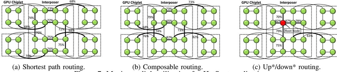
Figure 7: Maximum link utilization for HotSpot application.
