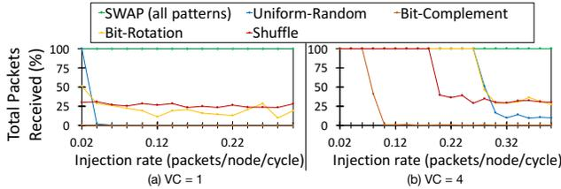
Figure 7: **Percentage of received packets when running a fully random routing algorithm. SWAP delivers all packets, irrespective of the traffic pattern. Without SWAP all traffic patterns see a sharp drop in delivered packets, due to deadlocks. The injection rate when deadlocks start depends on the traffic pattern and number of VCs.**
