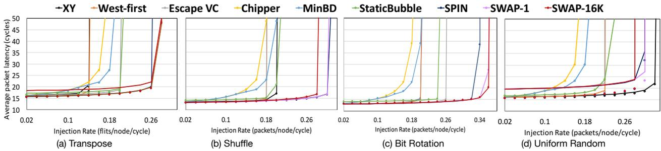
Figure 8: Performance of SWAP-K ( $K = \text{swapDutyCycle}$ ) with different traffic synthetic patterns, across deadlock-freedom techniques in a  $8 \times 8$  Mesh. Num VCs=4. Packet Size = Mix of 1 and 4 flits.
