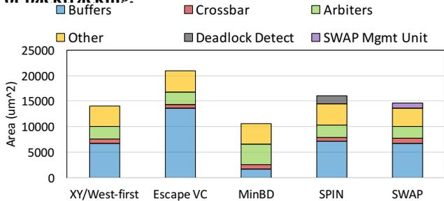
Figure 15: Post Place-and-Route Router Area (28nm TSMC, 1GHz).
