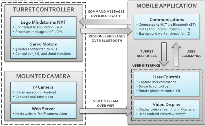
Figure 1 - Application Block Diagram
