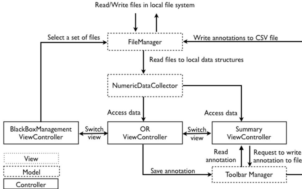
FIG 1. High-level block diagram.
