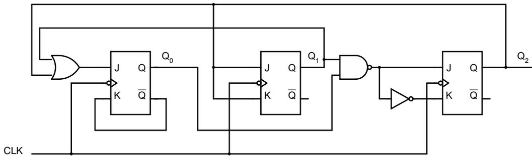
Draw a timing diagram (four complete clock cycles) for  $Q_0$ ,  $Q_1$  and  $Q_2$ . Assume that all initial values are 0. Note that all flip-flops are negative edge-triggered.
