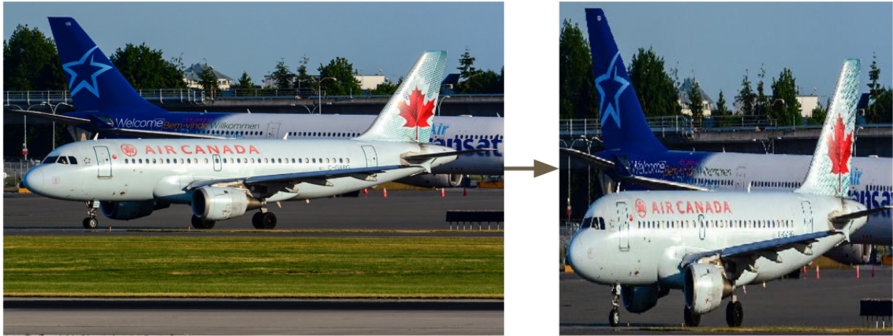
Figure 3: Example of a YOLO object identification model being used to intelligently crop the background out of photos as a data pre-processing step. The purpose of this is to remove unnecessary information before feeding the image into the neural network.
