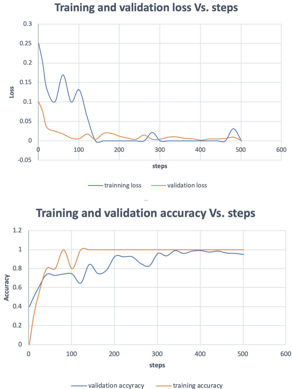
Figure 4. Plots of training and validation loss vs. # of steps (upper) as well as training and validation accuracy vs. # of steps (lower) when applying Triplet Net to CEDAR dataset
