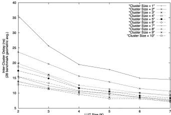
Fig. 17. Total intercluster delay for clusters of sizes 1–10.
