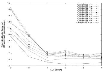
Fig. 15. Total intracluster delay for clusters of sizes 1–10.
