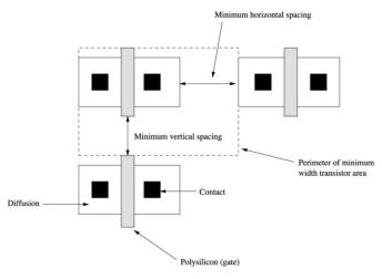
Fig. 4. Definition of a minimum-width transistor area [6].
