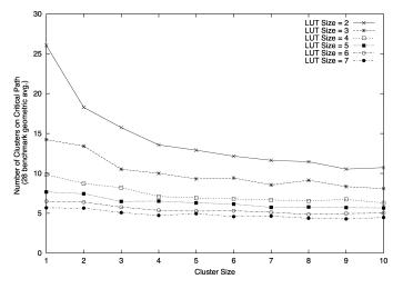
Fig. 18. Number of cluster levels on critical path.
