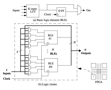
Fig. 2. (a) Structure of the basic logic element (BLE) and (b) logic cluster assuming a LUT size (K) of 4 [6].
