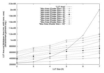
Fig. 11. Intracluster multiplexer area and LUT size.
