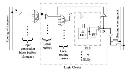
Fig. 5. Structure and speed paths of a logic cluster [6].
