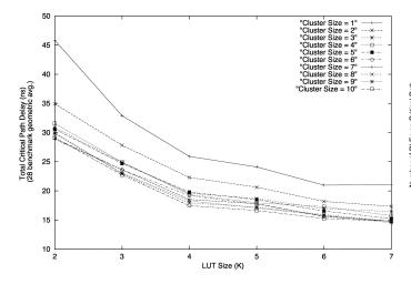
Fig. 14. Total delay for clusters of sizes 1–10.
