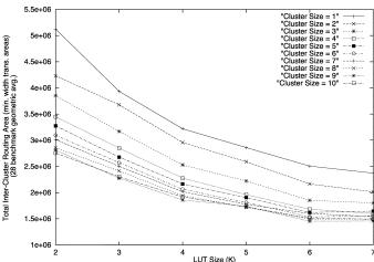
Fig. 12. Intercluster routing area.
