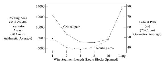
Figure 4: Speed and area of FPGAs vs. routing wire segment length.
