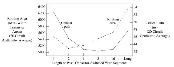
Figure 6: Comparison of FPGAs with 50% length 4 buffered and 50% pass-transistor-switched wires.
