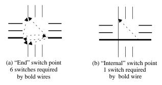
Figure 5: Switches required by a disjoint switch block at (a) end and (b) interior of wires.
