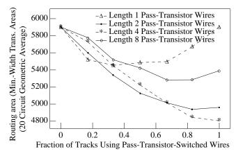
Figure 8: Area of FPGAs with a mix of length 4 buffered wires and pass-transistor-switched wires.
