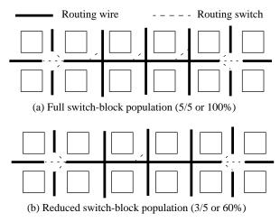
Figure 9: Examples of different switch-block population values.
