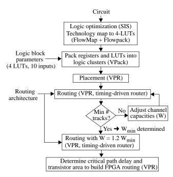
Figure 3: Architecture evaluation flow.
