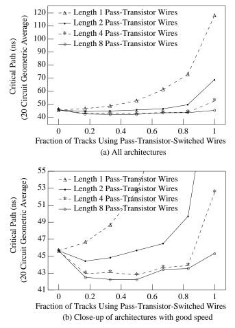
Figure 7: Speed of FPGAs with a mix of length 4 buffered wires and pass-transistor-switched wires.
