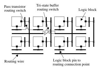
Figure 1: Example island-style FPGA routing architecture.
