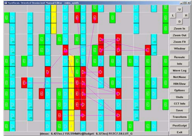
Figure 19 – 15 slowest paths in the Miim circuit
