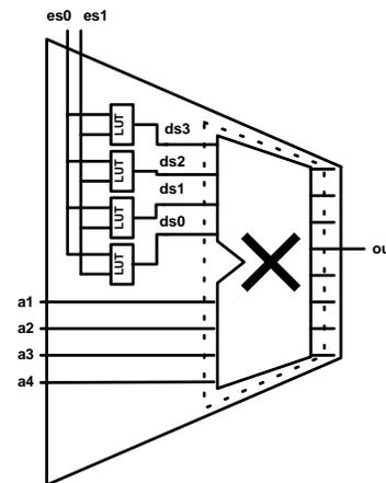
(b) Multiplexer built with an embedded multiplier
