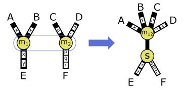
Fig. 3. A topology refinement step, which combines two Merge nodes and adds a Split node. The transmissions (x,y,p,q,r) routed over physical links (A-F) now face greater contention.
