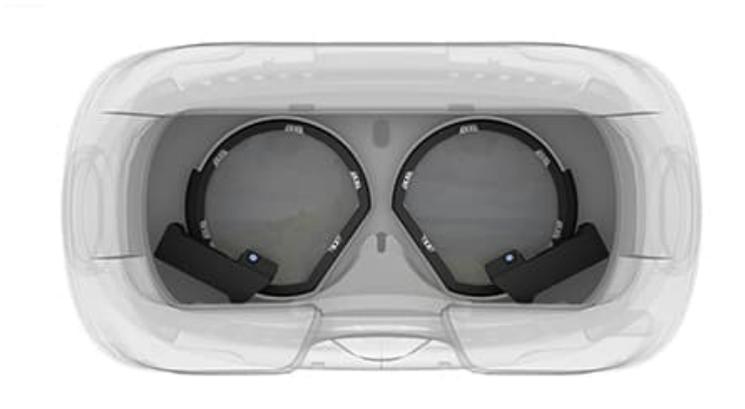
Figure 2.4: Pupil Labs Module inside the HTC Vive headset
