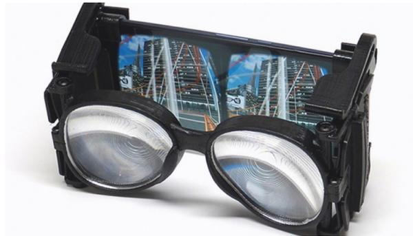
Figure 2.2: Lenses and Displays inside HTC Vive
