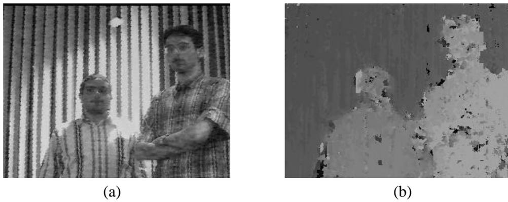
Figure 4.15 (a) Input from right camera, (b) Output disparity map
