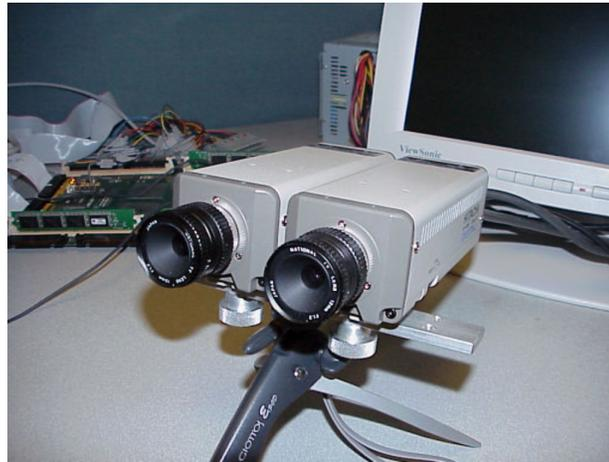
Figure 3.2: The camera head with two 1/2" CCD cameras. The focal length of the camera lenses is 12mm and the separation between the optic centers of the cameras is 70mm.
