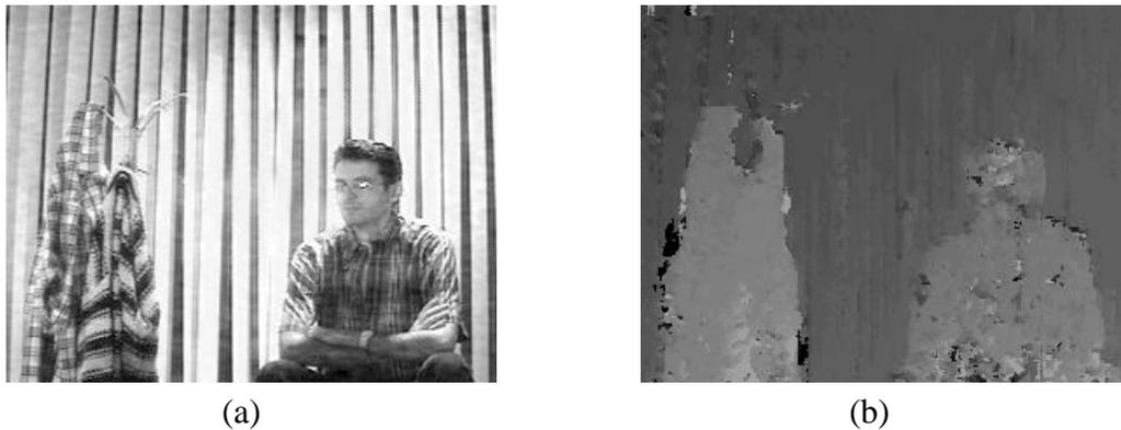
Figure 4.13: (a) Input from right camera, (b) Output disparity map
