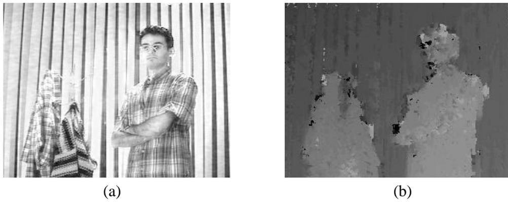
Figure 4.14 (a) Input from right camera, (b) Output disparity map
