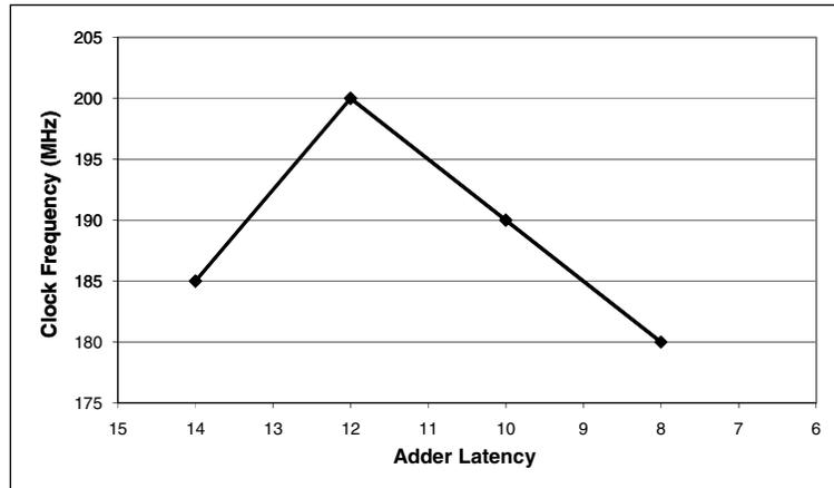
Fig. 7. Clock Frequency for Compute Engines with Different Adder Latencies on Stratix III 3SL340.
