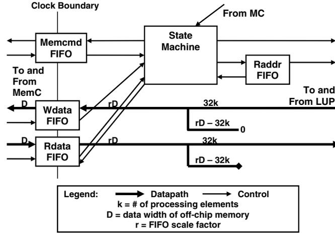
Fig. 4. Diagram of the Data Transfer Unit.
