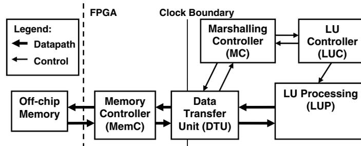
Fig. 2. Block diagram of Linear System Solver.
