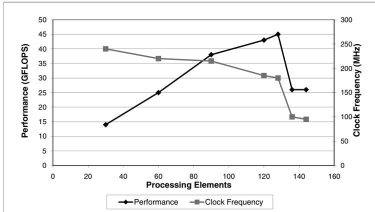
Fig. 6. The effect of varying the number of processing elements on performance and clock frequency on Stratix III 3SL340.
