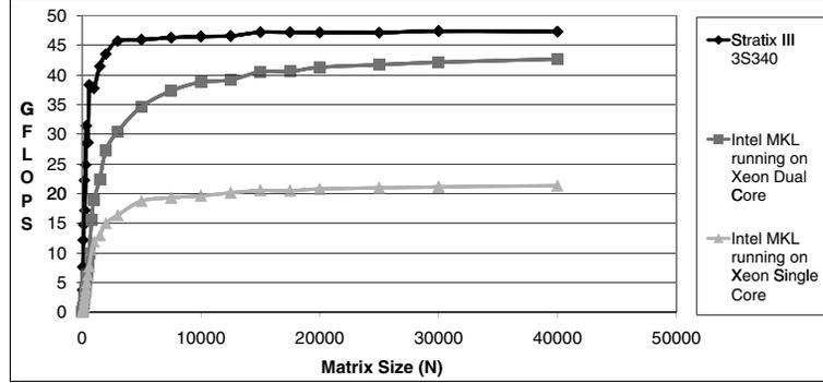
Fig. 8. Performance as a Function of Matrix Dimension.
