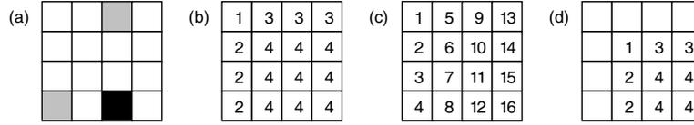
Fig. 1. (a) blocks required, in gray, to update the black block; (b) type of computation for each matrix block in the first block pass; (c) order of blocks updated in the first pass; (d) computation performed in the second block pass.
