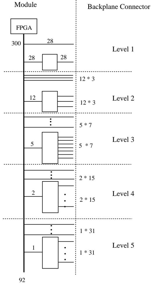
Figure 3.4 Routing Resource Distribution for 32 FPGA System
