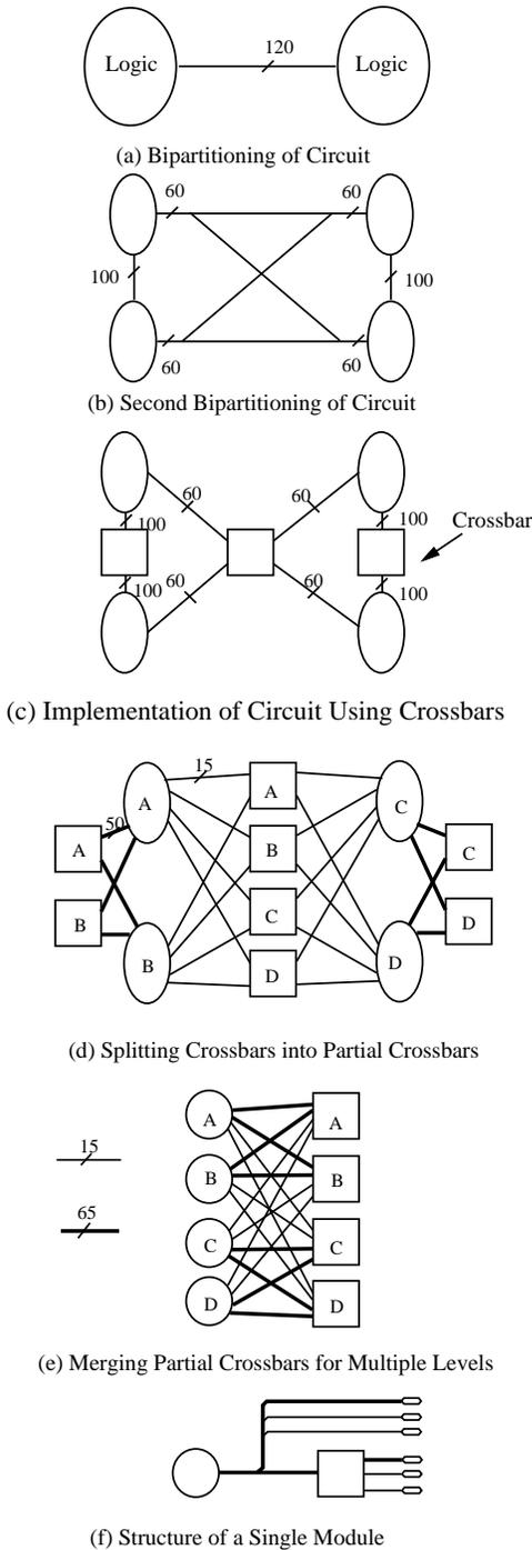
Figure 3.2 Construction of Non-uniform Partial Crossbar using Bipartitioning
