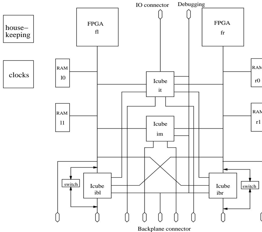
Figure 4.1 Organization of the TM-2 Printed Circuit Board
