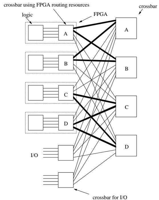
Figure 3.1 Partial Crossbar with Non-uniform Routing Density
