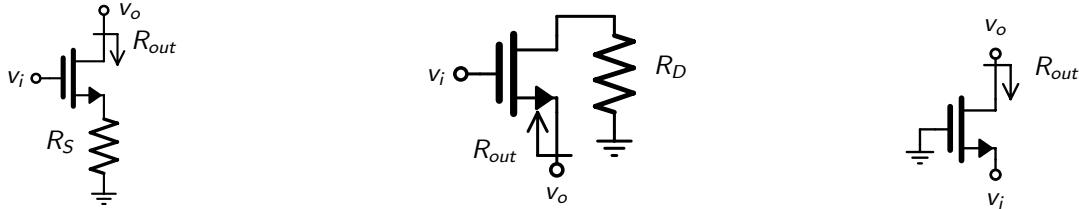
Accurate:  $R_{out} = r_o + (1 + g_m r_o)R_S$
