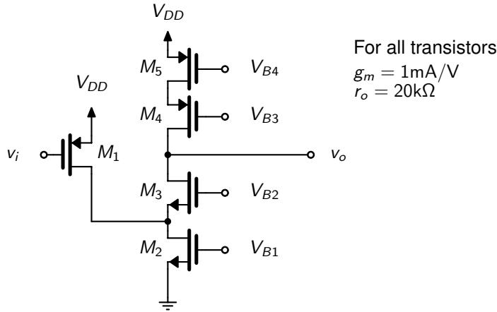
Find the small-signal output impedance,  $R_{out}$  and small-signal gain,  $v_o/v_i$ .
