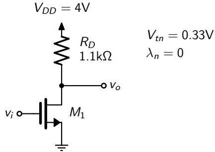
For the circuit above, when the dc bias voltage for  $v_i$  is 0.6V, then the measured dc voltage at  $v_o$  is 1.8V. Using the small-signal model, find the change in drain current,  $\Delta I_D$  when  $v_i$  goes from 0.6V to 0.63V
