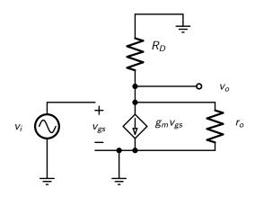
$$\begin{aligned} v_o &= -g_m v_{gs}(R_D||r_o) \\ v_{gs} &= v_i \\ v_o/v_i &= -g_m(R_D||r_o) \\ v_o/v_i &= -g_m * (R_D||r_o) = -(720e - 6) * ((1e3)||(46.3e3)) = -0.7048 \text{V/V} \end{aligned}$$
