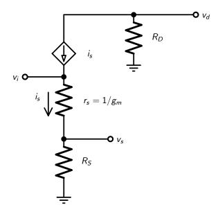
For  $v_s/v_i$ , there is a simple resistor divider between the applied voltage  $v_i$  and the measured output voltage  $v_s$ . As a result, we have
