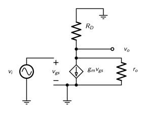
$$v_o = -g_m v_{gs}(R_D||r_o)$$
