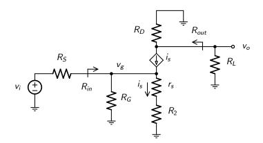
Since there is no current going into the gate of the transistor,
