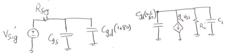
$$f_{in} = \frac{1}{2\pi C_{in} R_{sig}} = \frac{1}{2\pi (2 + (0.1)(1 + 80)) \times 20^k} = 788 \text{ Hz}$$
