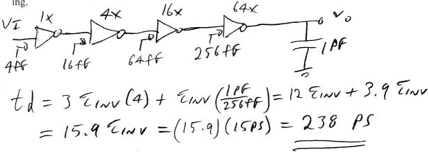
c) Explain why a fanout factor of 4 is generally used for inverter sizing in an inverter chain instead of a factor of e which was derived in class to be optimum. (hint: what was overlooked in the class derivation?)
