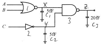
$$\begin{aligned} & \rho_{YN-1} &= \rho_{1} \Rightarrow_{0} f_{C_{1}} V_{00}^{2} \\ & \rho_{X=1} &= \rho_{A=0} \rho_{B=0} = (0.5)(0.6) = 0.3 \\ & \rho_{X=0} &= 1 - \rho_{X=1} = 0.7 \\ & \rho_{X(1\rightarrow 0)} &= (0.3)(0.7) = 0.21 \\ & \rho_{YN-1} &= (0.21)(1eq)(5e-15)(2.5)^{2} = 6.6 \mu W \\ & \rho_{YN-2} &= \rho_{1\rightarrow 0} f_{C_{2}} V_{00}^{2} = (0.3)(0.7)(1eq)(5e-15)(2.5^{2}) \end{aligned}$$
