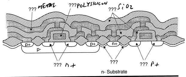
a) On the above diagram, label all the "???" signs with the material name (i.e. polysilicon, silicon dioxide, metal, p+, n+, p-, n-, etc.).
