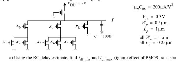
a) Using the RC delay estimate, find  $t_{df_{min}}$  and  $t_{df_{max}}$  (ignore effect of PMOS transistor).
