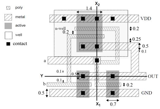
a) For the layout shown above, draw the schematic. Show the sizes of the NMOS and PMOS transistors. Also show the TOTAL drain area,  $A_D$ , and TOTAL drain perimeter,  $P_D$ , attached to the OUT node.
