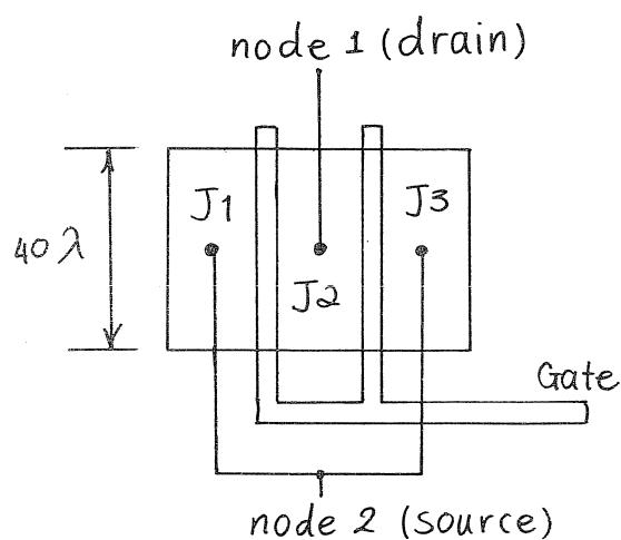
$$\therefore C_{db} = A_{J_2}C_j + P_{J_2}C_{jsw} = \underline{0.016 \text{ pF}}$$
