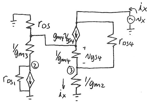
$$V_{GS4} = V_{G4} - V_{S4} = V_2 \times \frac{r_{DS}}{V_{gm3} + r_{DS}} - V_3$$
