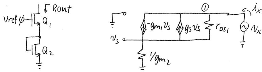
Use test voltage,  $V_x$ , to find  $R_{out}$ .
