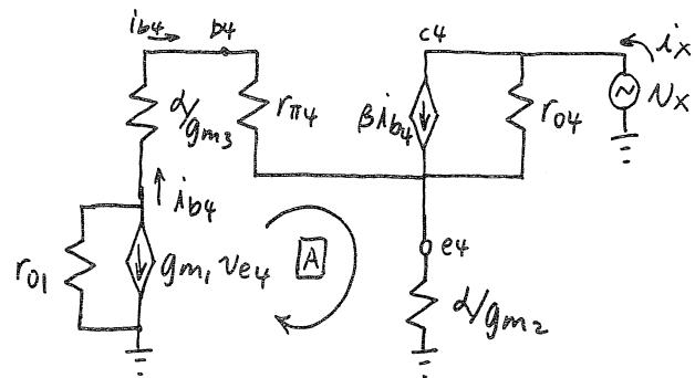
$$\text{KCL at output: } i_x - \beta i_{b4} - (N_x - N_{e4})/r_{04} = 0 \quad \boxed{1}$$
