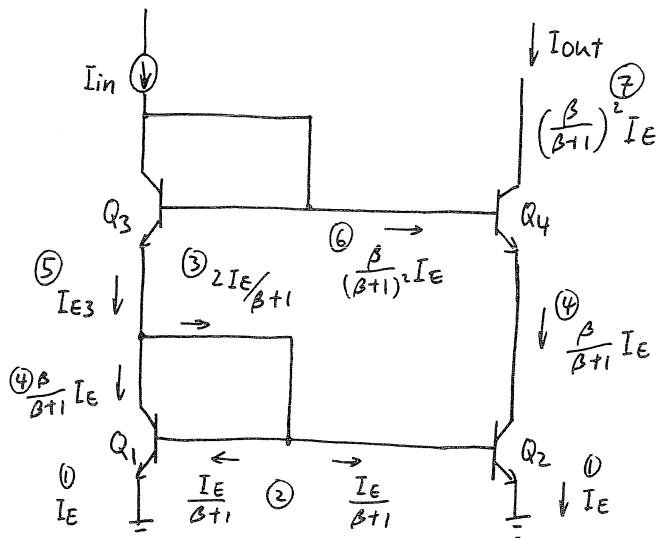
$$\textcircled{1} \quad \because V_{be1} = V_{be2}, \\ \therefore I_{E1} = I_{E2} \stackrel{\Delta}{=} I_E$$
