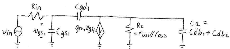
$$M_{3dB} \approx \frac{1}{R_{in}[C_{gs1} + C_{gd1}(1 + g_m R_2)] + R_2(C_{gd1} + C_2)}$$
