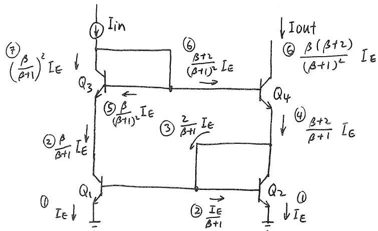
$$\begin{aligned} (1) \quad & \because V_{be1} = V_{be2} \\ \therefore I_{E1} &= I_{E2} \stackrel{A}{=} I_E \end{aligned}$$
