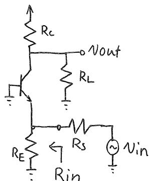
Find  $\frac{V_{out}}{V_{in}}$  and  $R_{in}$
