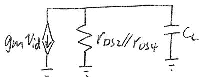
$$W-3dB = \frac{1}{r_{DS2} // r_{DS4} \times C_L} \\ = \frac{1}{154 \times 10^3 \times 100 \times 10^{-12}} \\ = \underline{2\pi \times 10 \text{ kHz}}$$
