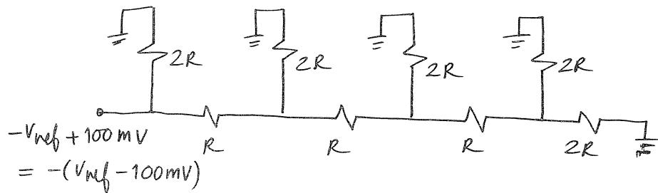
In effect,  $V_{ref}$  has decreased by  $100\text{mV}$  and the circuit still operates as if there is no voltage drop across the switches.
