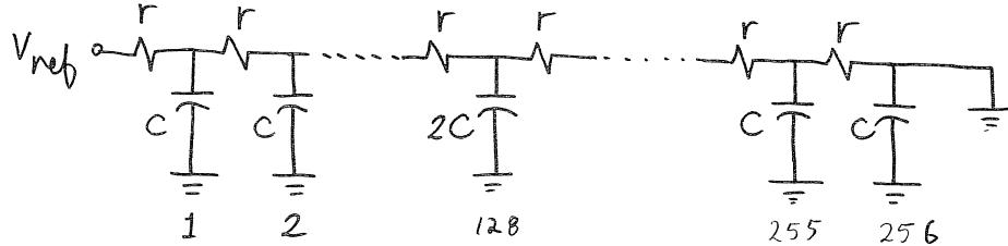
In the equivalent circuit shown,  $r = \frac{400}{256} \Omega$ ,  $C = 0.1 \mu F$ .
