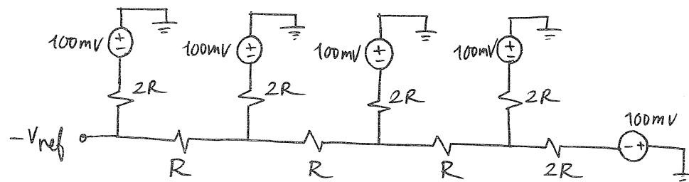
The 100-mV voltage sources model the voltage drop of the switches. One end of  $2R$ -resistor is connected to  $-100\text{mV}$ . Therefore, they can all be connected together and the  $100\text{mV}$  voltage-source can be moved and added to the  $V_{ref}$  source. This will not change the current calculations of  $2R$ -resistors.
