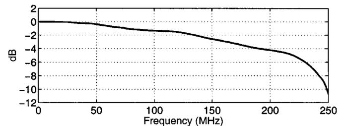
Fig. 8. Line driver frequency response:  $f_{-3\text{dB}} = 160$  MHz.
