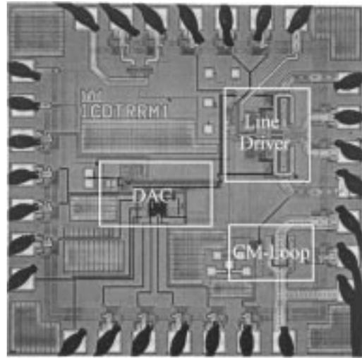
Fig. 7. Chip photomicrograph.
