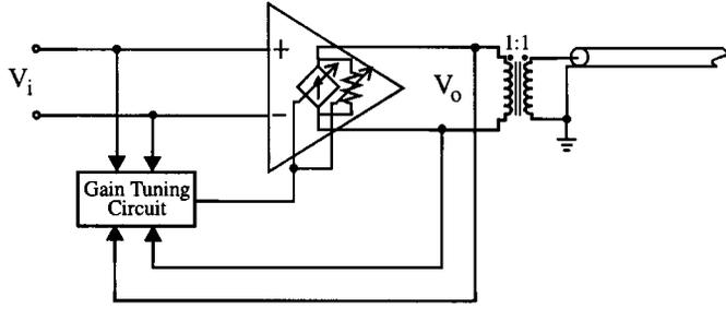
Fig. 2. Proposed line driver topology block diagram.
