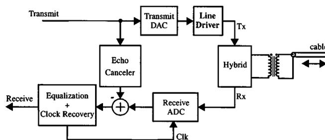
Fig. 1. The main blocks of a transceiver.
