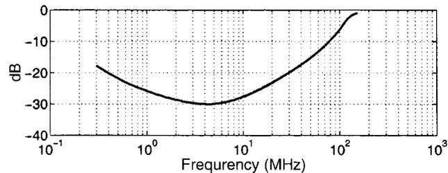
Fig. 12. Return loss performance including transformer.
