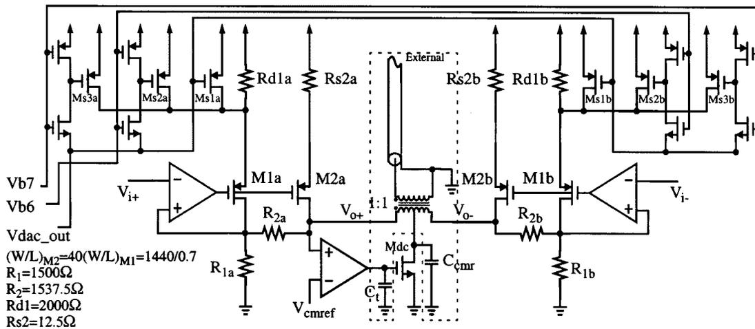
Fig. 5. Complete differential line driver.
