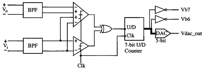
Fig. 6. SS-LMS gain tuning circuit.
