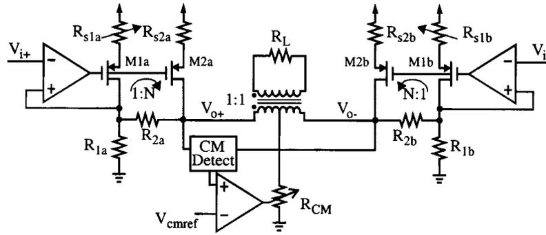
Fig. 4. Transformer-coupled differential driver topology.
