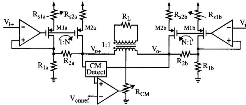
Fig. 4. Transformer-coupled differential driver topology.
