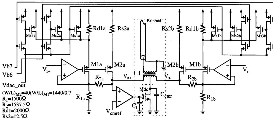
Fig. 5. Complete differential line driver.
