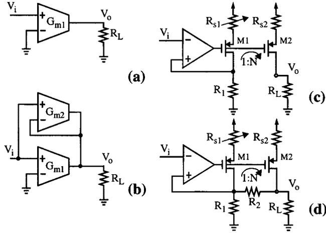
Fig. 3. Circuit for driving low resistive loads.
