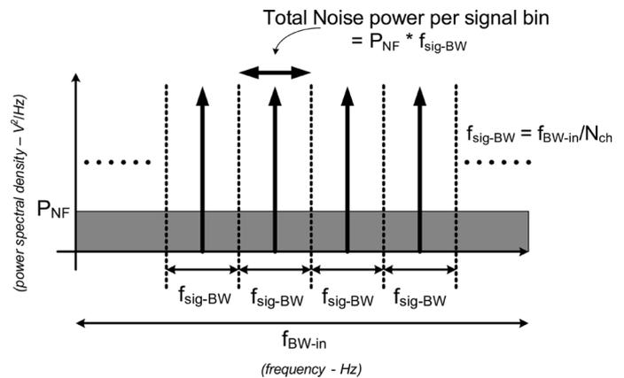
Fig. 1. Example OFDM spectrum.
