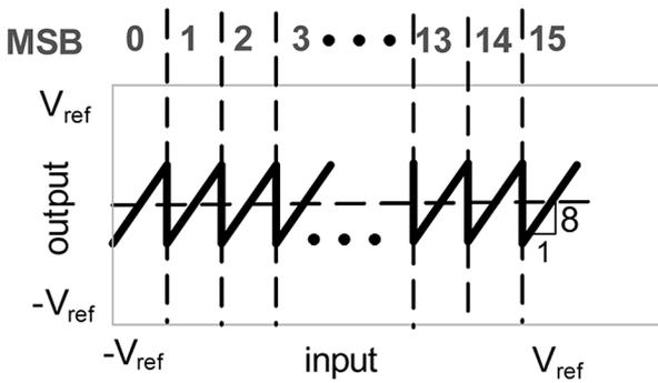
Fig. 7. Ideal residue transfer curve of 4-bit pipeline stage.
