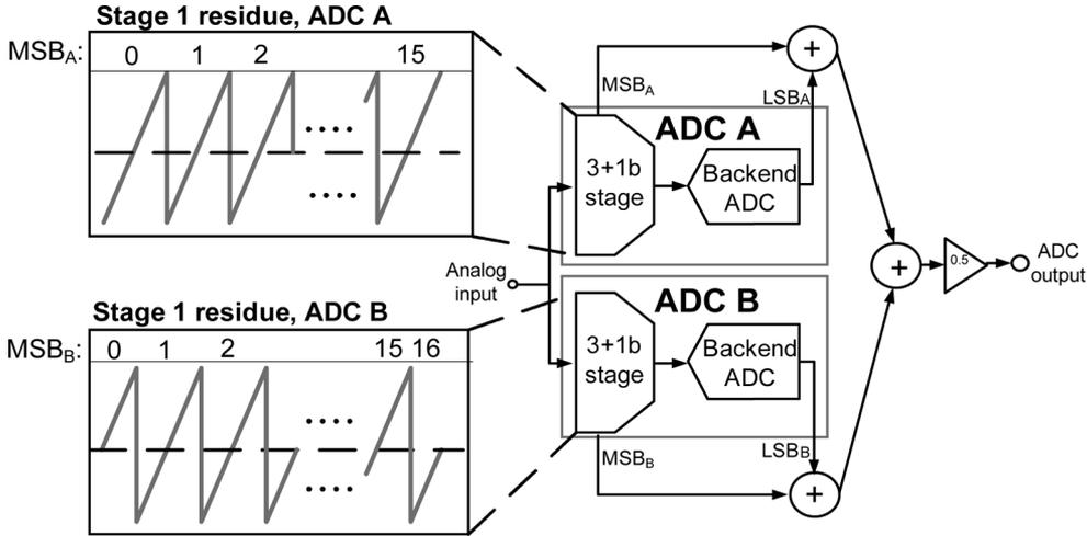
Fig. 10. Dual ADC topology of this work.
