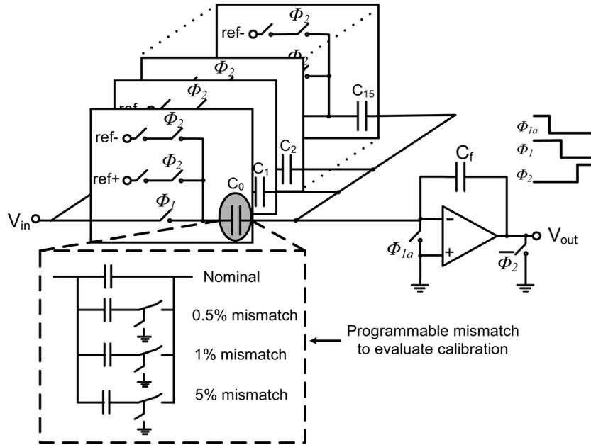
Fig. 18. Topology of first stage MDAC (implemented fully differentially in this work).
