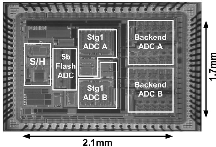
Fig. 22. Micrograph of fabricated IC in 1.8 V 0.18  $\mu\text{m}$  CMOS.
