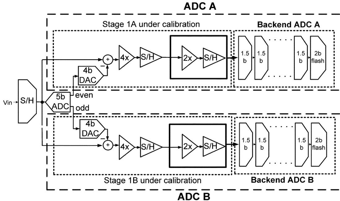
Fig. 15. Analog portion of ADC topology in detail.
