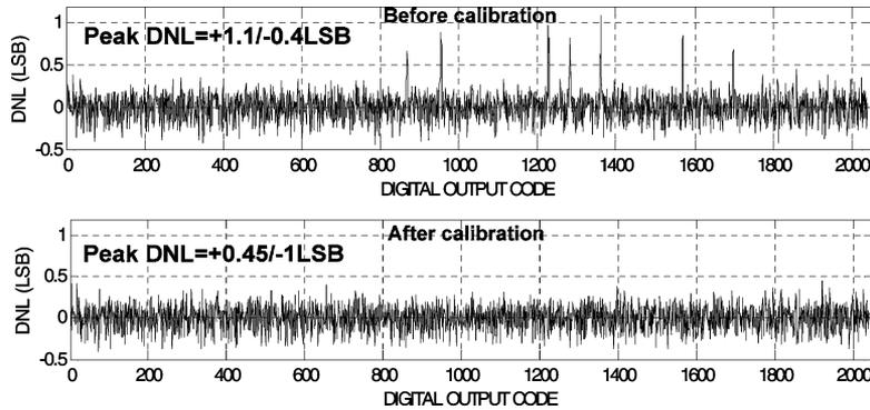
Fig. 24. DNL before and after calibration.
