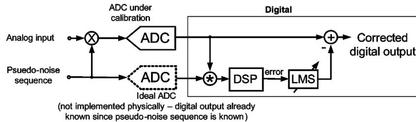
Fig. 3. Principle of background calibration.
