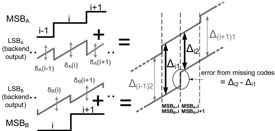
Fig. 12. Transfer curves of key ADC outputs with gain, DAC errors included.
