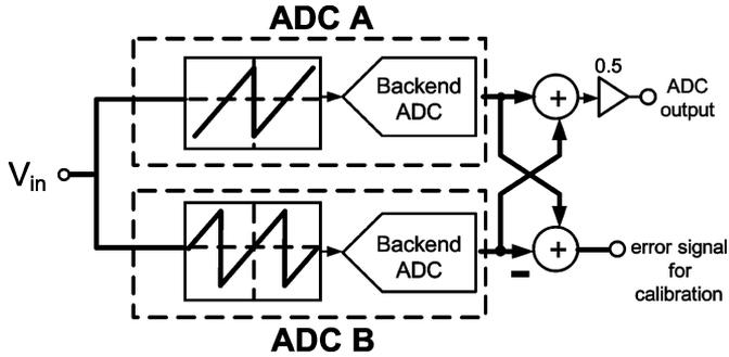
Fig. 4. Example split-ADC topology.
