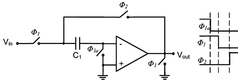
Fig. 16. Sample and hold topology (implemented fully differentially in this work).
