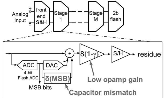
Fig. 5. Pipeline topology, first stage shown in detail including error sources.
