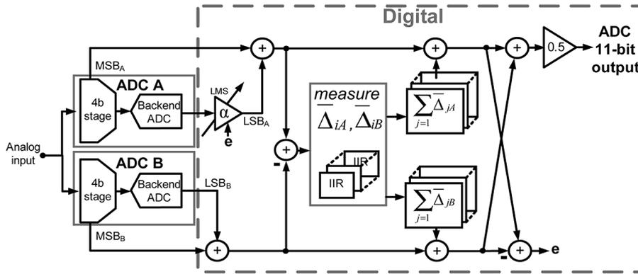
Fig. 14. Full ADC topology of this work.
