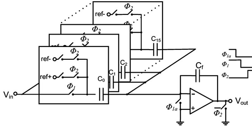
Fig. 6. Example implementation of 4-bit MDAC (shown single-ended, implemented differentially in practice).
