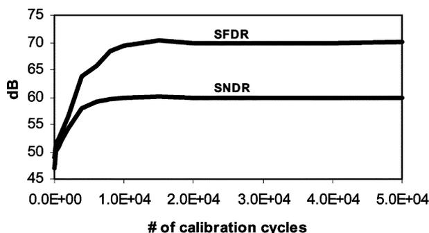
Fig. 27. ADC SNDR, SFDR improvement with number of calibration cycles.
