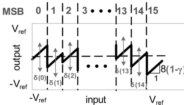
Fig. 9. Residue transfer curve showing impact of DAC and gain errors.
