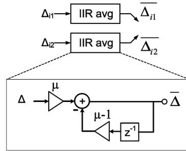
Fig. 20. Detail of IIR filter blocks used in “estimate error” block of Fig. 21.
