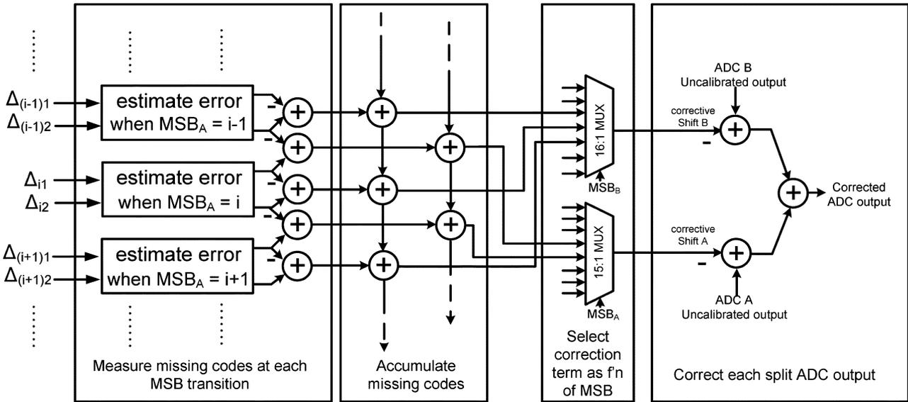
Fig. 21. Digital implementation of calibration.
