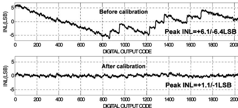
Fig. 23. INL before and after calibration.
