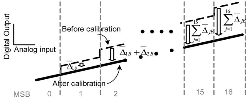
Fig. 13. Illustration of how correction terms for ADC B are derived from estimates of missing codes (correction topology of ADC A is similar).
