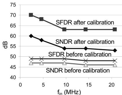
Fig. 26. Variation of ADC SNDR, SFDR with input frequency, before and after calibration.
