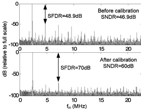
Fig. 25. FFT of ADC output before and after calibration.
