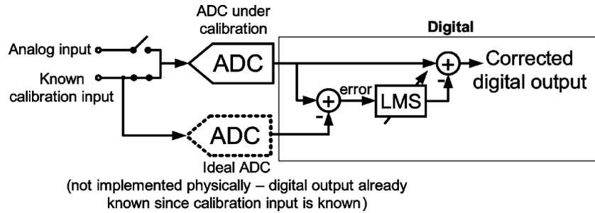
Fig. 2. Principle of foreground calibration.
