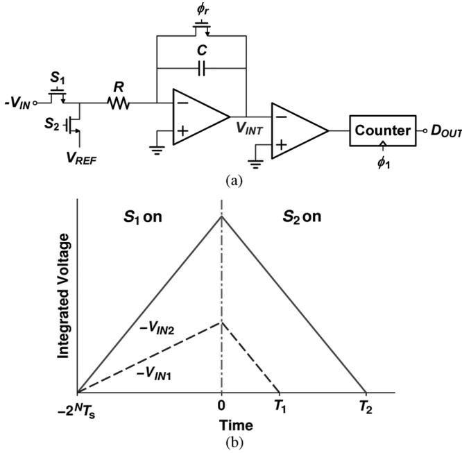
Fig. 2. Dual-slope A/D converter. Two sample input voltages are shown with their respective digital outputs  $T_1$  and  $T_2$ .  $\phi_1$  is operating at the sampling frequency  $f_s$ . (a) Architecture. (b) Integrator output.
