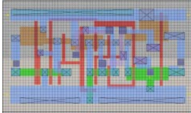
Figure 5.10: Cell haf001 after migrated towards TSMC 0.18\mu m technology.
