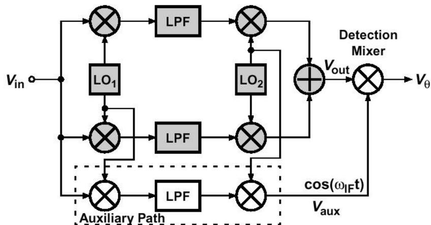
Figure 7 – Generation of the Phase Error Signal [2]
