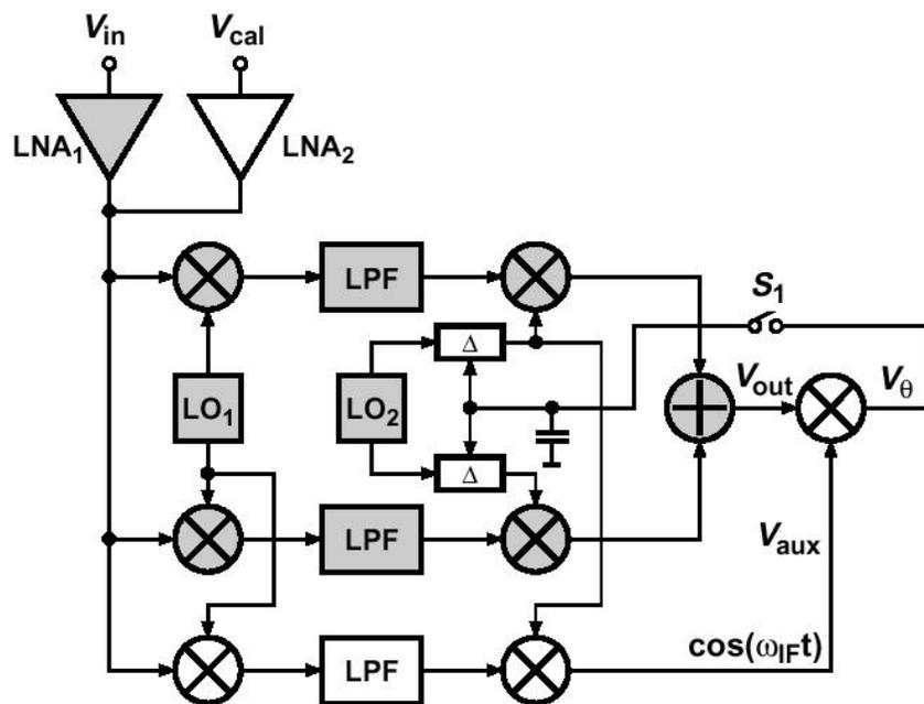
Figure 8 – Image-Reject Receiver with Phase Calibration Loop [2]
