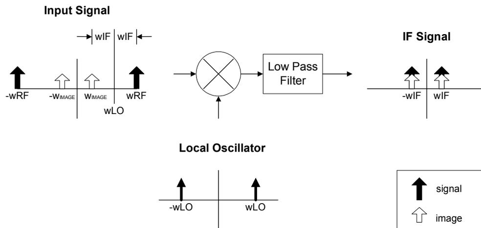
*Figure 2 – Image Corruption of Desired Signal due to Mixing Operation*
