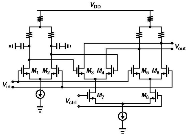
Figure 11 – Variable Delay Cell [2]
