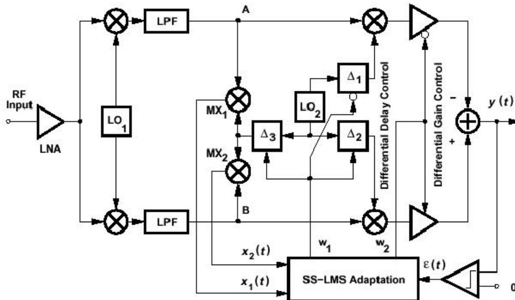
Figure 9 – Image-Reject Receiver with SS-LMS Calibration [3]
