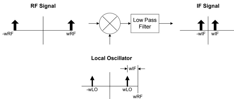
*Figure 1 – Function of an Analog Mixer*
