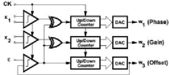
Figure 10 – SS-LMS Adaptation Circuit [3]
