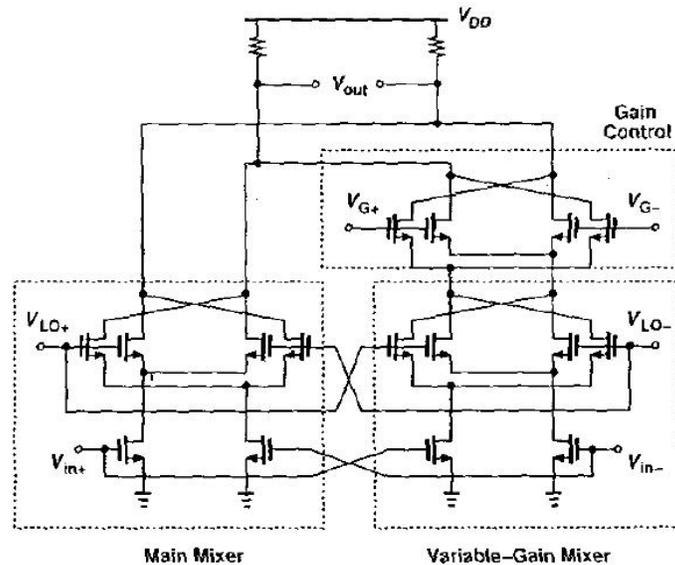
Figure 12 – Variable Gain Cell [3]
