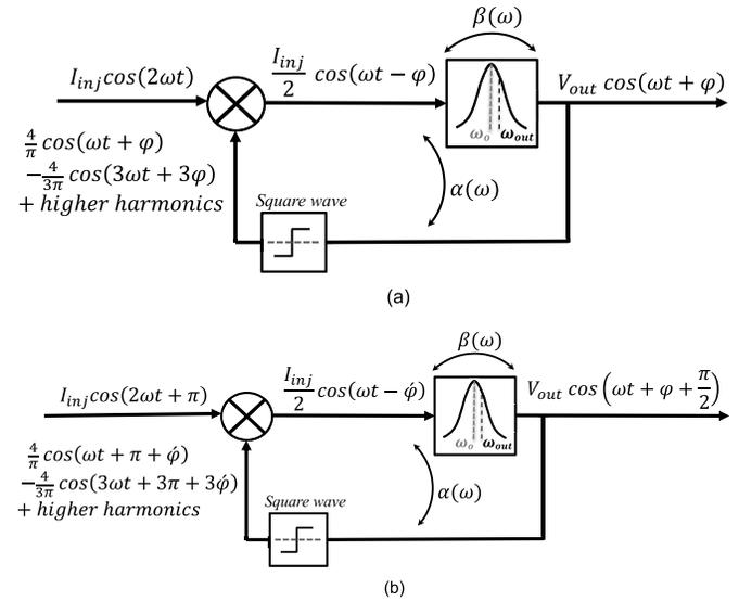
Fig. 2. Simple behavioral model for the ILFD. (a) No input phase shift [12], (b) With  $180^\circ$  input phase shift.
