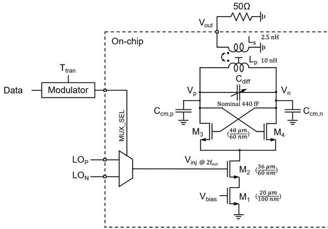
Fig. 11. Schematic of the proposed transmitter. The multiplexer and injection-locked power amplifier are ON-chip. The multiplexer selection signal is generated in software. External LOs are used as inputs.
