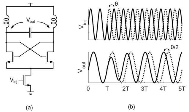
Fig. 1. (a) Injection-locked LC frequency divider with tail injection. (b) Injected signal and corresponding output voltage for an unmodulated (dotted line) and modulated (solid line) input [9].
