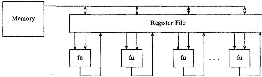
Figure 1. Block Diagram of an Ideal VLIW Execution Engine
