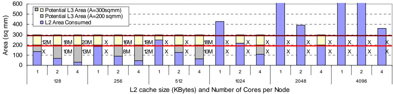
Figure 2. Area Considerations for a 32-Core LCMP Cache Design.
