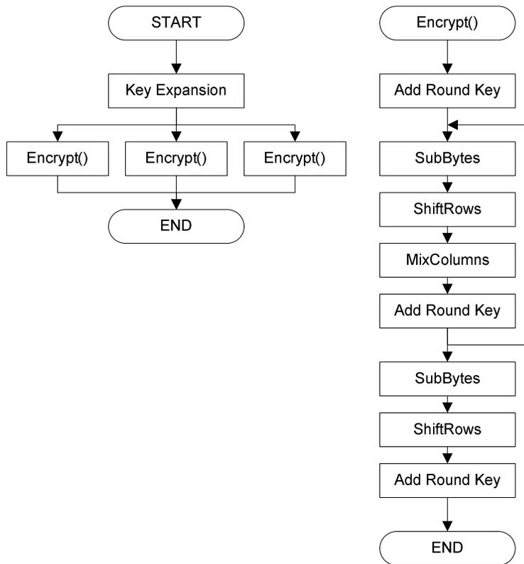
**Figure 2 - Parallel AES Algorithm**
