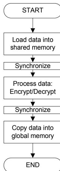
**Figure 3 - Thread Execution Stages**
