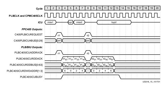
Figure 2-10: ISPLB Non-Pipelined Non-Cacheable Sequential Fetch
