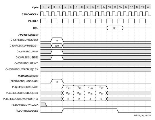
Figure 2-26: DSPLB 2:1 Core-to-PLB Line Read
