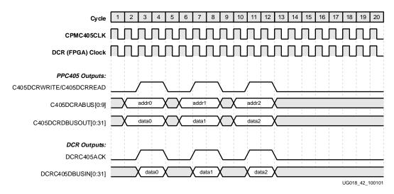
Figure 2-33: DCR Interface Mode 0, 1:1 Clocking, Combinatorial Acknowledge
