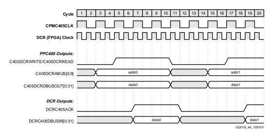
Figure 2-35: DCR Interface Mode 0, 1:2 Clocking, Latched Acknowledge
