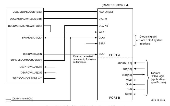
Figure 3-2: DSOCM to BRAM Interface: 8K Example
