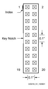
Figure A-2: Trace-Connector Physical Layout
