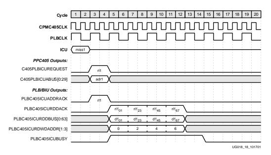
Figure 2-12: ISPLB 2:1 Core-to-PLB Line Fetch
