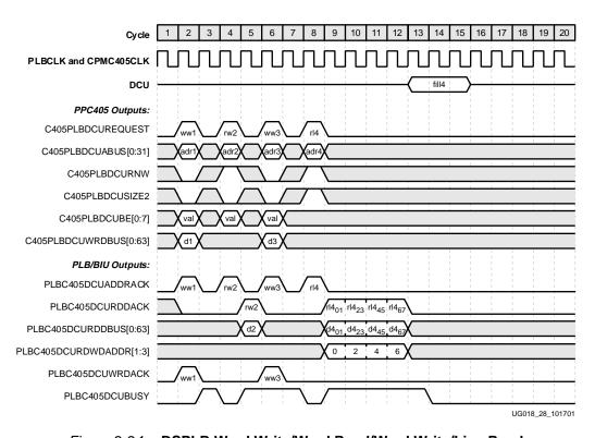
Figure 2-24: DSPLB Word Write/Word Read/Word Write/Line Read
