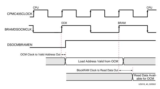
Figure 3-6: Multi-Cycle Static Performance Analysis of DSOCM (Load Operation)
