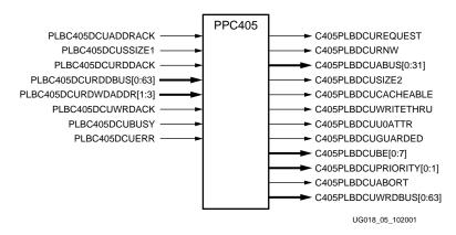
Figure 2-15: Data-Side PLB Interface Block Symbol
