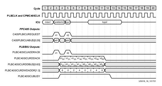
Figure 2-11: ISPLB Pipelined Non-Cacheable Sequential Fetch
