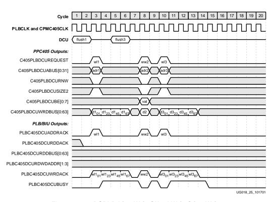
Figure 2-21: DSPLB Line Write/Word Write/Line Write
