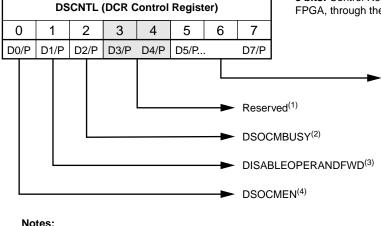
8 bits: Control Register for DSOCM. They are also configurable via FPGA, through the DSCNTLVALUE inputs to the processor block.
