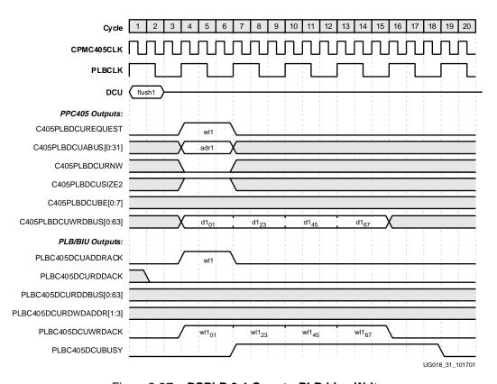
Figure 2-27: DSPLB 3:1 Core-to-PLB Line Write
