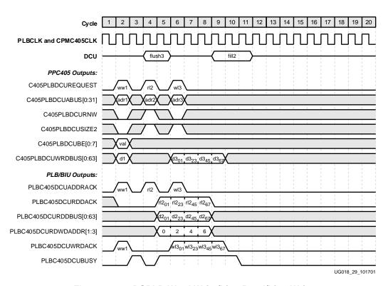
Figure 2-25: DSPLB Word Write/Line Read/Line Write
