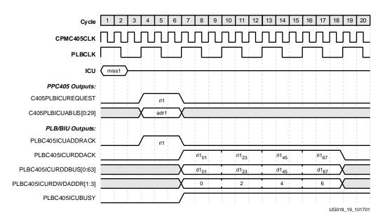
Figure 2-13: ISPLB 3:1 Core-to-PLB Line Fetch
