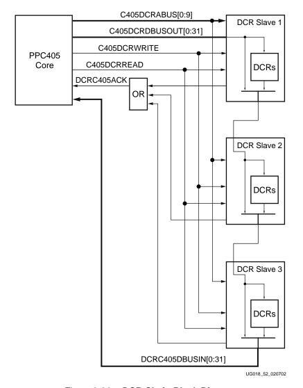
Figure 2-29: DCR Chain Block Diagram
