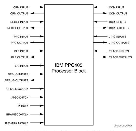
Figure C-1: PowerPC 405 Processor Block (Simplified)
