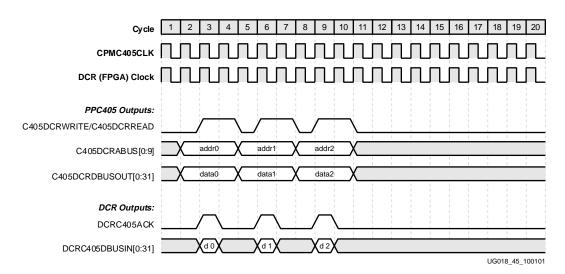
Figure 2-36: DCR Interface Mode 1, 1:1 Clocking, Combinatorial Acknowledge
