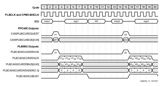
Figure 2-6: ISPLB Non-Pipelined Cacheable Seguential Fetch (Case 1)
