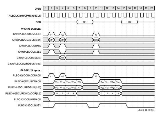
Figure 2-18: DSPLB Line Read/Word Read/Line Read
