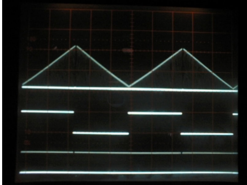
Figure 4.5: Measured linearity of the computational array configured for signed multiplication on each cell (XOR configuration). Two cases are shown: binary weight storage elements are all actively charged, and all discharged. Waveforms shown are, top to bottom : the analog voltage output on the sense line; input data (in common for both input and weight shift register); and input shift register clock.
