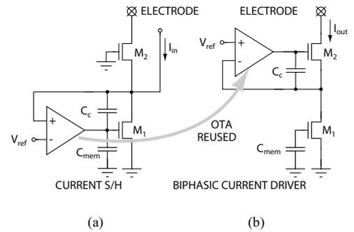
Fig. 4. Circuit implementation of the neural stimulator. (a) Current storing phase, and (b) current driver phase.
