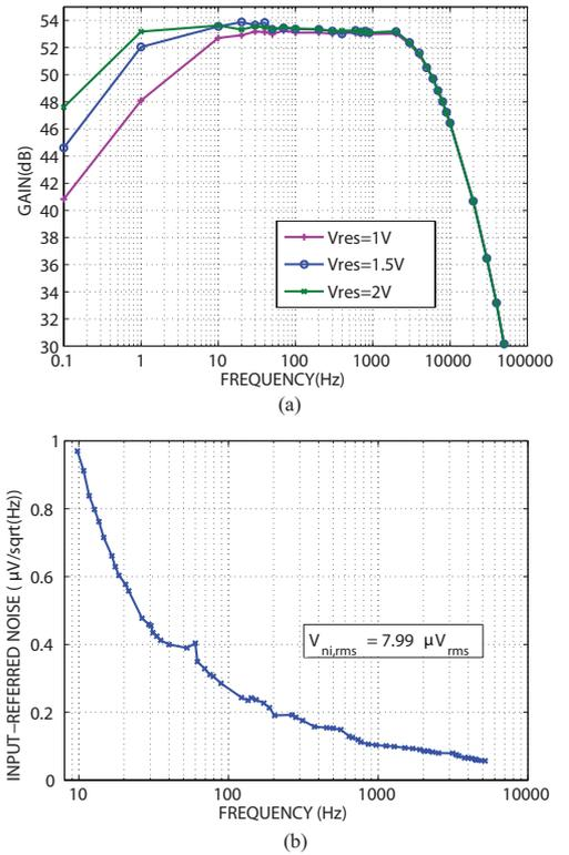
Fig. 6. (a) Experimentally measured amplitude frequency response of the neural amplifier. (b) Experimentally measured noise of the neural amplifier.
