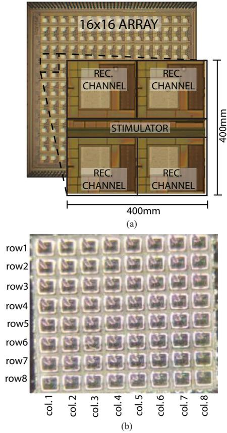
Fig. 5. (a) Micrograph of the  $0.35\mu\text{m}$  CMOS prototype. (b) Top view of a Utah electrode array (UEA) bonded onto the CMOS die. UEA shanks connect to every fourth recording channel and each stimulation channel.
