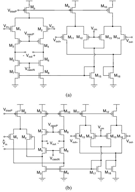
Fig. 3. (a) Telescopic amplifier in the first stage of the recording channel. (b) Folded-cascode amplifier in the second stage of the recording channel.
