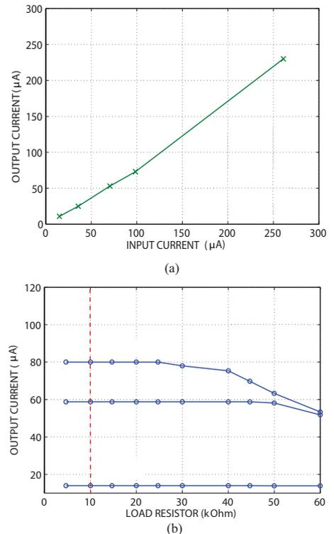
Fig. 7. (a) Experimental neural stimulator transfer characteristic. (b) Experimental neural stimulator output current for a varying load.
