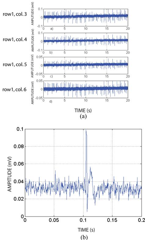
Fig. 8. (a) Neural activity in a mouse hippocampus recorded by the chip through four on-chip UEA electrodes. (b) One neural spike from (a).
