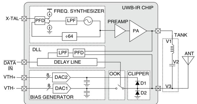
Fig. 1. Block diagram of the proposed UWB-IR transmitter.
