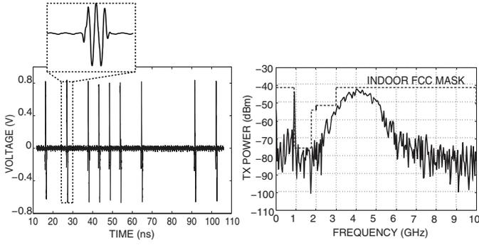
Fig. 5. Experimentally measured modulated time domain output of the transmitter (left), and power spectrum (right).
