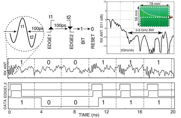
Fig. 6. Receiving antenna return loss, and experimentally measured output of the receiving antenna by oscilloscope (Agilent DSO-92004) (top), rise and fall edges, and data stream detected by computer algorithm processing the RX antenna signal.
