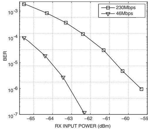
Fig. 8. Experimentally measured TX-RX bit error rate.
