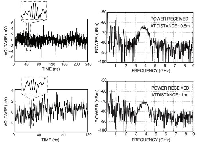
Fig. 7. Experimentally measured received UWB signal by antenna at 50cm (top) and 1m (bottom).
