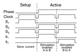
Fig. 4. Timing diagram for implementing a biphasic stimulus.
