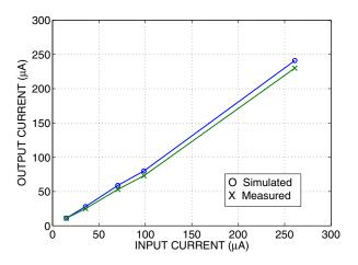
Fig. 7. Transfer characteristic of the current driver for  $10k\Omega$  load.
