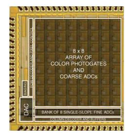
Fig. 5. Micrograph of the 0.35  $\mu$ m standard CMOS 2 mm×2 mm color sensor die with a 175  $\mu$ m×175  $\mu$ m pixels.
