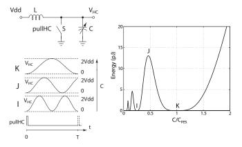
Fig. 4. Lossless LC oscillator with variable load capacitance C and examples of three corresponding  $V_{HC}(t)$  waveforms (left). Energy dissipation in switch S of a lossless varying-capacitance LC oscillator (right).
