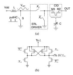
Fig. 3. (a), LC tank oscillator driving an array of charge-recycling CID cells. One cell is shown, with two charge-coupled MOS transistors M2 and M3 according to Fig. 1 and Fig. 2. (b), double-range input-enabled energy recovery logic (ERL) driver.
