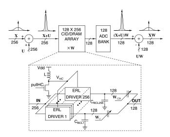
Fig. 5. Mixed-signal array and stochastic modulation architecture.
