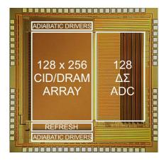
Fig. 6. Adiabatic VMM processor micrograph and floor plan. The die area is  $2.2 \times 2.2 \text{mm}^2$ .
