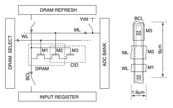
Fig. 1. CID/DRAM computational array, with 3-T unit cell and with peripheral functions (left). Compact, single-pitch layout of the cell (right).
