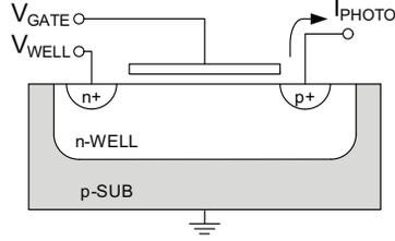
Fig. 2: Spectrally-sensitive photodiode (SPD) inspired by [6], modified for a p-type substrate.
