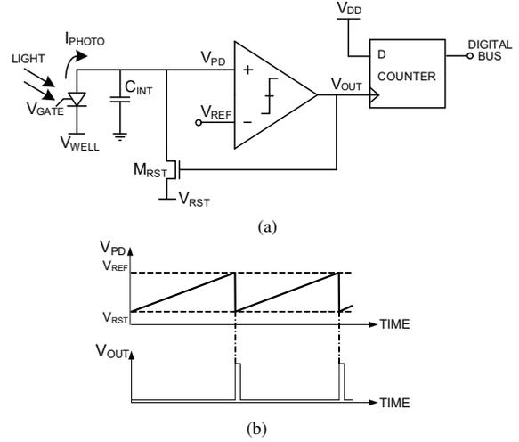
Fig. 3: FCS implementation. (a) FCS circuit with current-to-frequency ADC. (b) Voltage transients under illumination.
