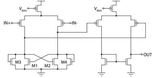
Fig. 4: The voltage comparator.
