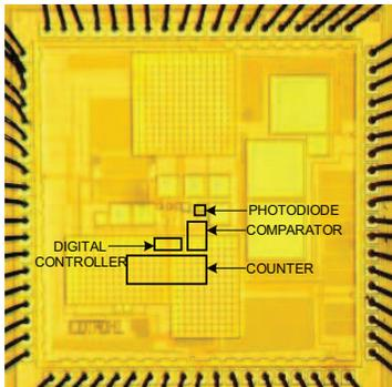
Fig. 6: Chip micrograph of the field-modulated color sensor.
