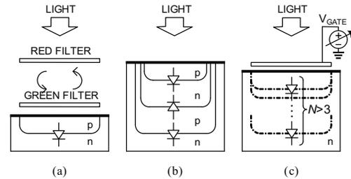
Fig. 1: Evolution of spectral imaging approaches. (a) Classical method of mechanically switching between optical filters. (b) Buried triple p-n-junction embedding diodes at three fixed depths. (c) Photo sensing region depth modulation enabling light collection at multiple electronically-tunable depths [6].
