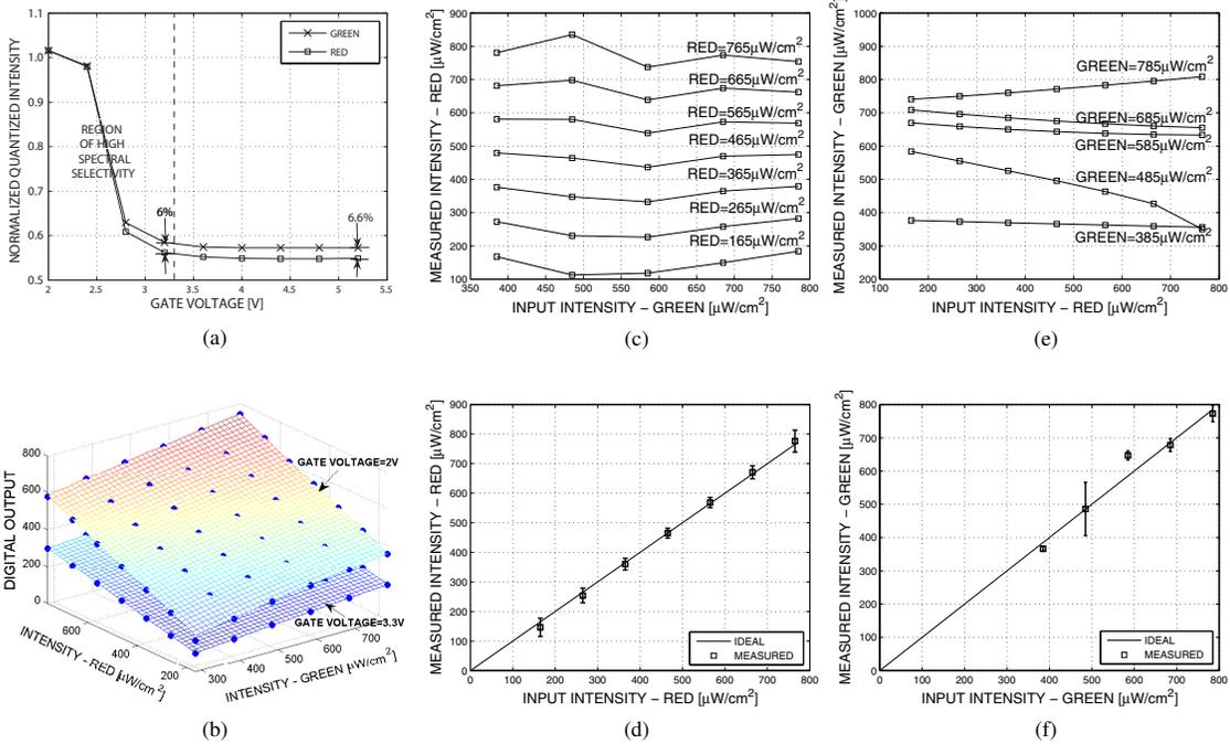
Fig. 5: Experimental results. (a) Measured photo response of the FCS normalized at  $V_{GATE} = 2\text{V}$ . (b) Measured photo responses of the FCS across gate voltages and illumination. (c) Measured intensity at discrete red (640nm) levels across green (540nm) levels. (d) Measured vs. input intensity at 640nm. (e) Measured intensity at discrete green levels across red levels. (f) Measured vs. input intensity at 540nm.
