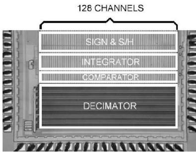
Fig. 7. Micrograph of the 128-channel algorithmic  $\Delta\Sigma$ -modulated FIR filter. To demonstrate the advantages of the approach to large-scale sensory signal processing, the FIR filters are integrated with a  $128 \times 128$ -pixel array, not shown, as part of a mixed-signal focal-plane processor.
