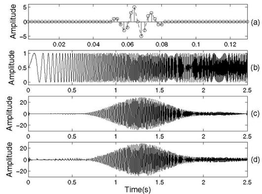
Fig. 8. (a) 15-tap integrated Morlet wavelet. (b) Sinusoidal input signal with frequency increasing linearly in time. (c) FIR Filter response computed by a floating-point processor. (d) FIR filter response, experimentally computed and measured from a single channel of the VLSI  $\Delta\Sigma$ -modulated FIR filter array.
