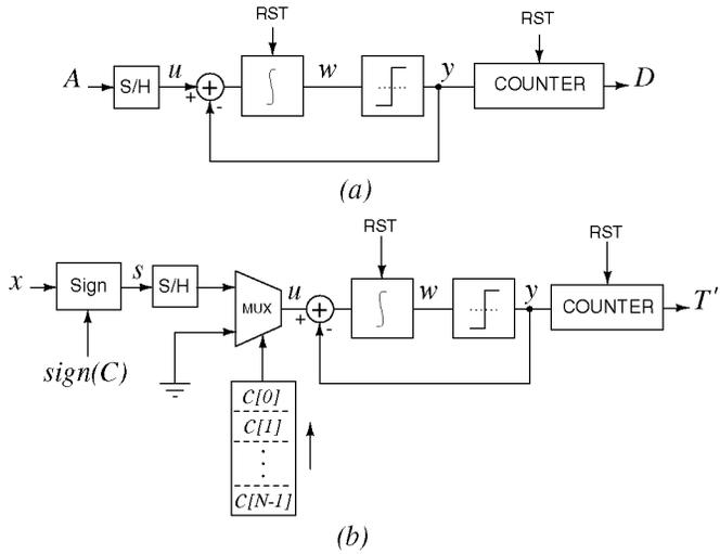
Fig. 2. (a) First-order  $\Delta\Sigma$  incremental A/D converter. (b)  $\Delta\Sigma$ -modulated multiplying ADC.
