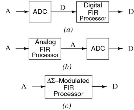
Fig. 1. FIR filter architectures with (a) a digital processor, (b) an analog processor, and (c) a  $\Delta\Sigma$ -modulated processor.
