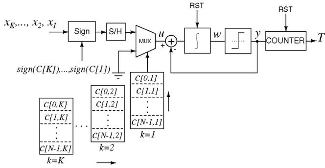
Fig. 4.  $\Delta\Sigma$ -modulated weighted averaging ADC.
