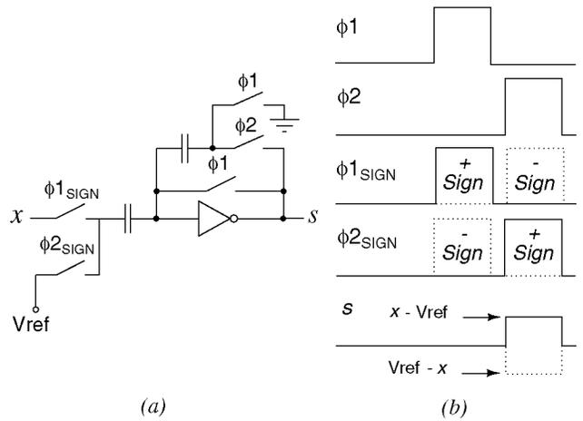
Fig. 3. (a) The sign unit circuit in the  $\Delta\Sigma$ -modulated FIR filter. (b) Sign circuit timing diagram; for a continuous range of signed outputs,  $V_{\text{ref}} = \min\{x\}$ . The circuit also performs the sample-and-hold operation. (S/H is explicitly shown in Figure 2(b) for clarity.)
