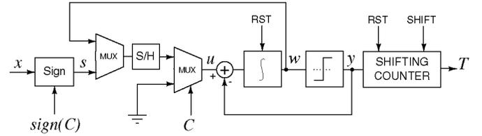
Fig. 6. Algorithmic  $\Delta\Sigma$ -modulated FIR ADC, with residue resampling across the integrator, and shifting counter for the decimator.
