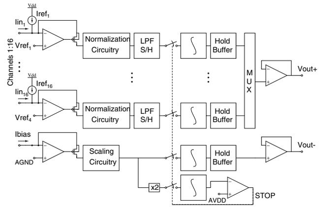
Fig. 1. Block diagram of the current-acquisition integrated neural interface.
