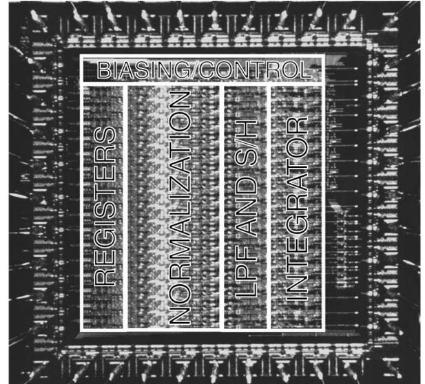
Fig. 2. Chip micrograph of the 16-channel integrated track-and-hold potentiostat. Die size is 2.25  $\times$  2.25 mm<sup>2</sup> in 1.2  $\mu$ m CMOS technology.
