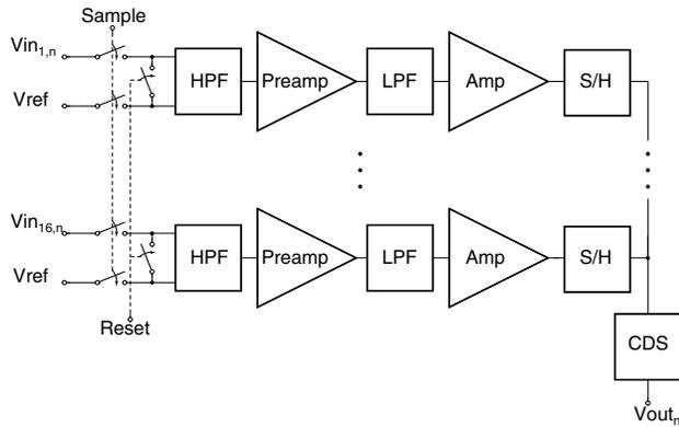
Fig. 3. Block diagram of one column of the voltage-acquisition integrated neural interface.
