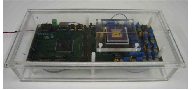
Fig. 10. Fluidic chamber attached to the top of the testing printed circuit board.
