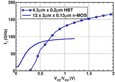
Fig. 3 Drain/collector voltage dependence of  $f_T$  in 130-nm n-MOSFETs and SiGe HBTs.
