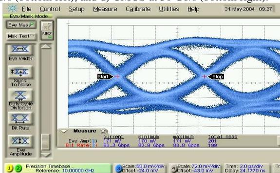
Fig.6: 80-Gb/s output eye of SiGe BiCMOS 2:1 MUX.
