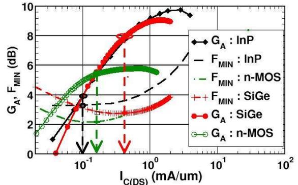
Fig. 2  $F_{MIN}$  and associated gain as a function of bias current at 36 GHz for 130-nm n-MOSFETs, SiGe and InP HBTs.
