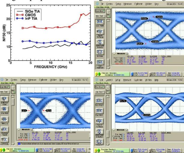
Fig. 5: a) (top left) Noise figure and eye diagrams of b)(top right) SiGe HBT comparator at 40Gb/s, c) InP comparator at 40 Gb/s (bottom left), and d) CMOS at 30 Gb/s (bottom right).
