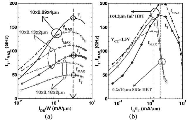
Fig.1 Measured  $f_T$  and  $f_{MAX}$  as a function of drain/collector current for a) 180-nm, 130-nm, and 90-nm n-MOSFETs, and b) for SiGe and InP HBTs [12].
