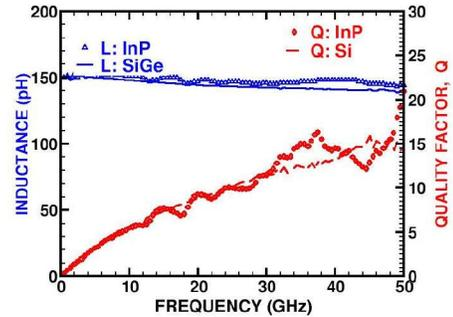
Fig. 4 Measured  $L$  and  $Q$  of Si and InP inductors.
