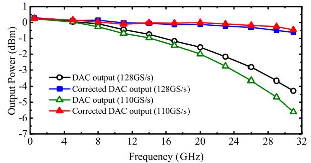
Fig. 15. Simulated large signal DAC bandwidth.
