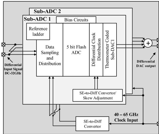
Fig. 2. ADC block diagram.
