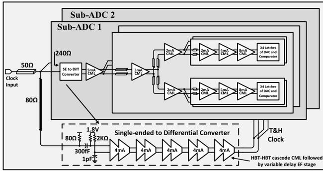
Fig. 11. Block diagram of the clock distribution network.
