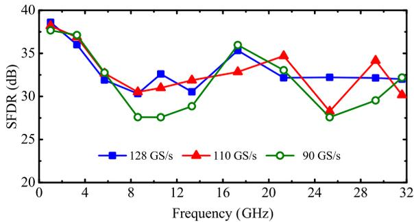
Fig. 20. SFDR measurements for different sampling rates and input signals up to 32 GHz.
