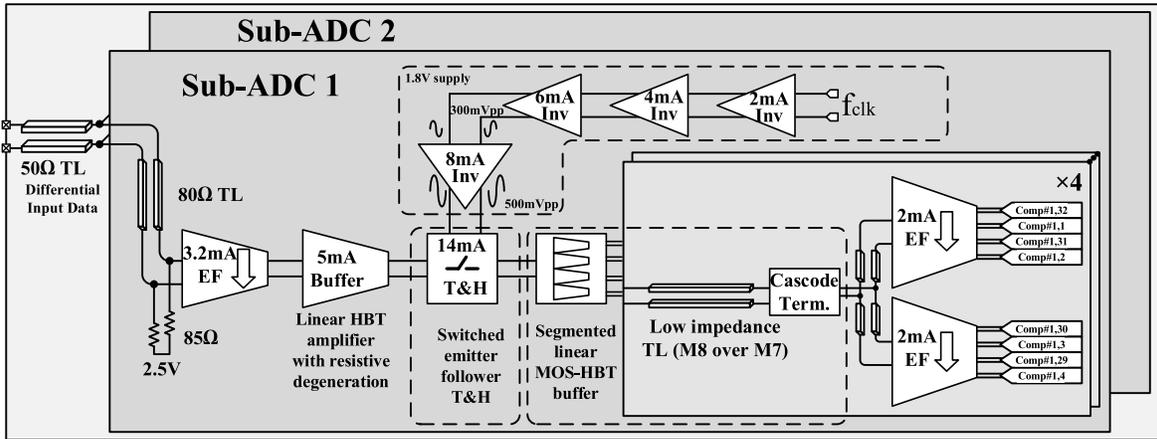
Fig. 7. Block diagram of the analog input signal sampling and distribution network in each sub-ADC.
