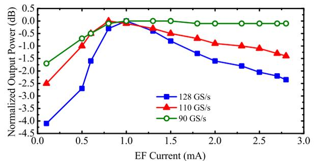
Fig. 24. Impact of the bias current in the EF delay cell on the normalized output power of the ADC for a 31.6-GHz input signal for different sampling rates.
