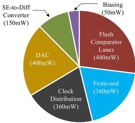
Fig. 17. Breakdown of the power consumption of the ADC-DAC chip.
