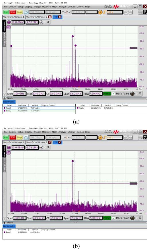
Fig. 26. DAC output spectrum for a 31.3-GHz input signal sampled at 128 GS/s (a) with and (b) without intentional mismatch between the two sub-ADCs.
