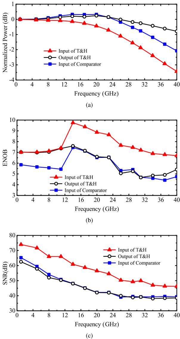
Fig. 13. Simulation of the input analog signal sampling and distribution tree. (a) Normalized power. (b) ENOB. (c) SNR.
