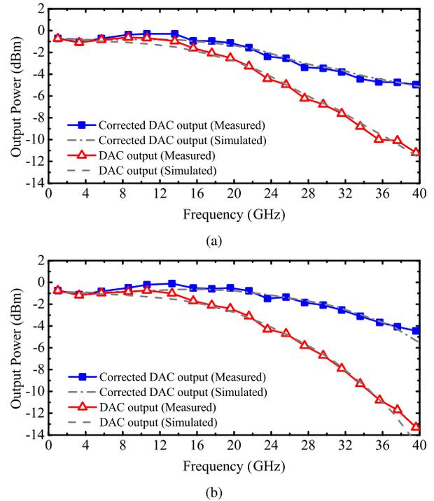
Fig. 25. Comparison of the measured and simulated large signal output power of the ADC-DAC combo versus analog input signal frequency at (a) 128 and (b) 110 GS/s.
