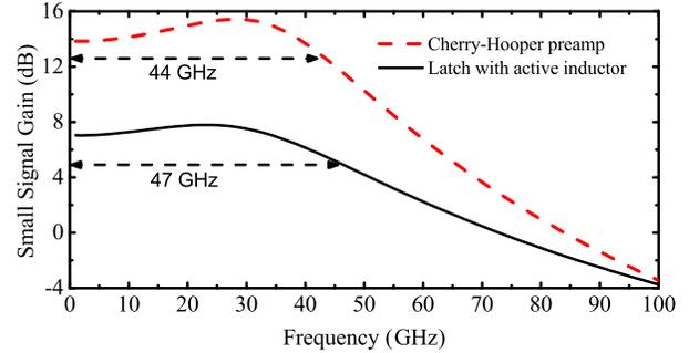
Fig. 6. Small-signal simulation of the preamplifier and comparator latch bandwidths.
