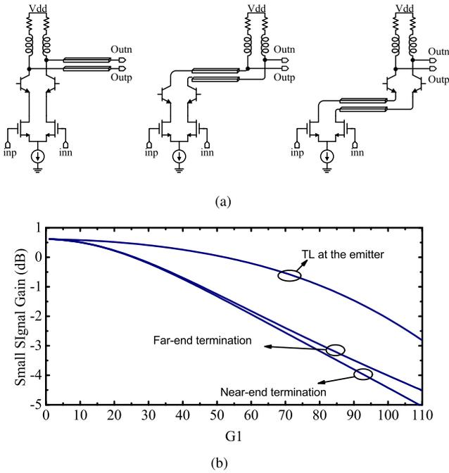
Fig. 9. Performance comparison for the different MOS-HBT buffer configurations. (a) Schematics. (b) Small-signal simulation.
