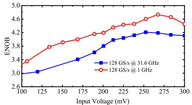
Fig. 23. Measured ENOB at 128 GS/s as a function of the input signal peak-to-peak voltage per side at 1 and 31.6 GHz.
