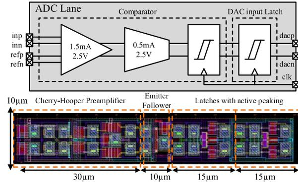
Fig. 3. Latched comparator lane schematic and layout.
