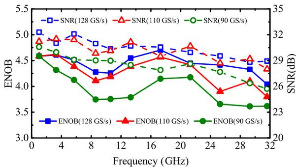
Fig. 21. ENOB and SNR measurements for different sampling rates and input signals up to 32 GHz.
