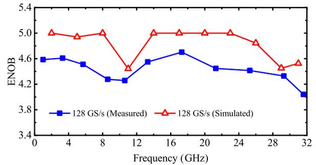
Fig. 22. Comparison of simulated and measured ENOB at 128 GS/s for input signals up to 32 GHz.
