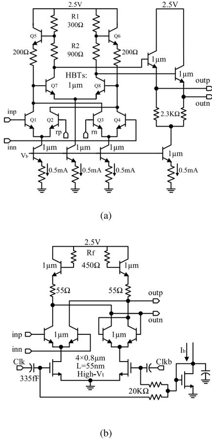
Fig. 4. Schematic of building blocks in ADC comparator lanes. (a) Cherry-Hooper preamplifier followed by EF stage. (b) Quasi-CML latch with active peaking.
