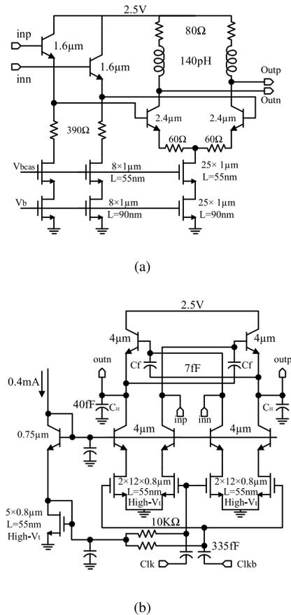
Fig. 8. Schematic of building blocks in signal sampling and distribution network. (a) Input buffer. (b) Track and hold amplifier.
