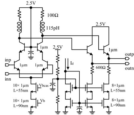
Fig. 12. Schematic of the cells in single-ended-to-differential converter. The current in the EF stage is varied externally to adjust the delay.
