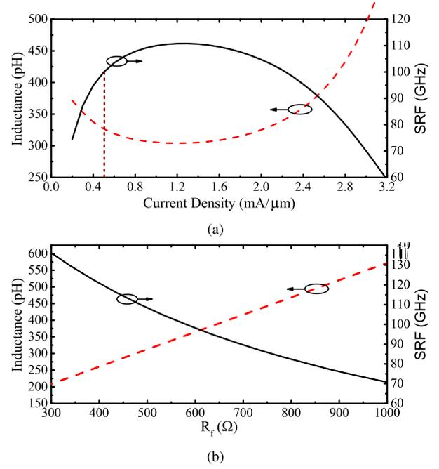
Fig. 5. Simulation of the active inductor design space: inductance and self-resonance frequency as a function of (a) HBT current density per emitter width and (b) peaking resistor value,  $R_f$ .
