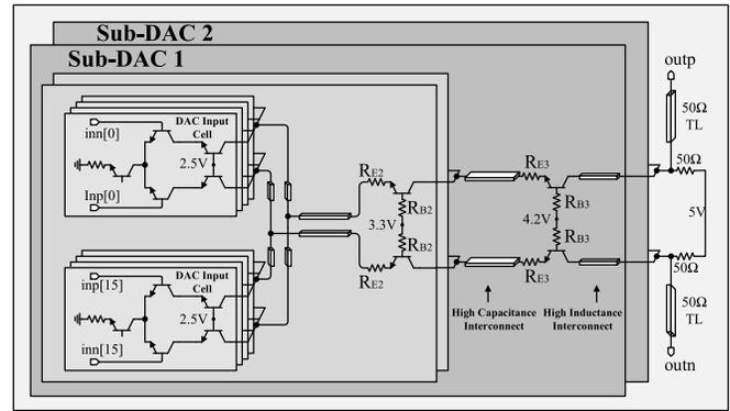
Fig. 14. DAC schematic.
