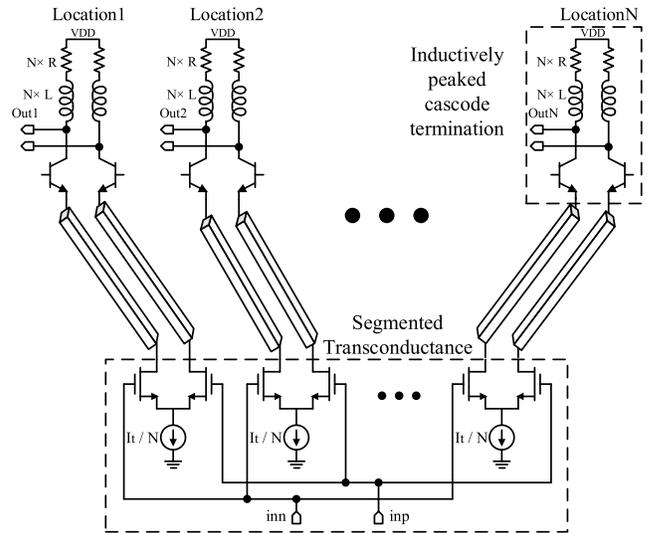
Fig. 10. Sampled analog input signal distribution buffer with segmented transconductance.
