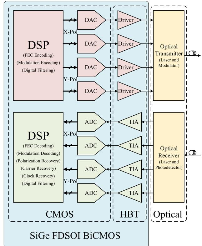
Fig. 1. Block diagram of a dual-polarization fiber-optic system with 16-QAM or higher order modulation.
