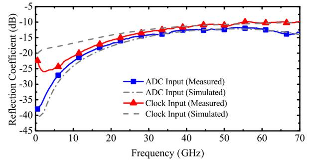
Fig. 18. Reflection coefficient of the ADC analog signal and clock inputs.
