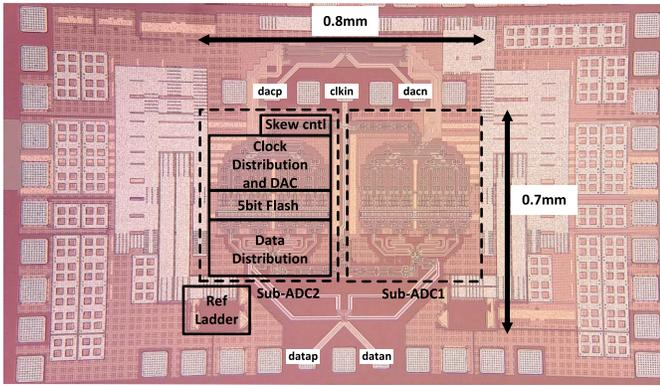
Fig. 16. ADC chip microphotograph showing the layout of the sub-ADC in the inset.
