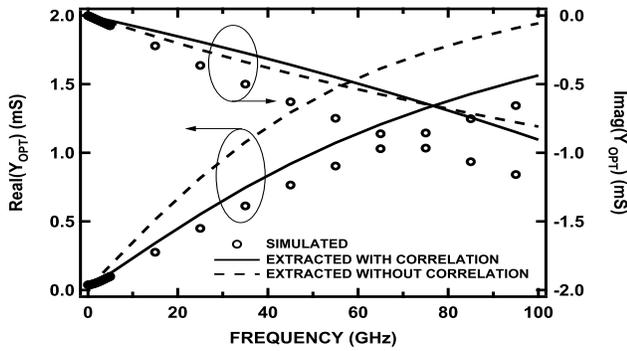
Fig. 5. Simulated and extracted  $Y_{OPT}$  with and without correlation at minimum noise bias. The emitter area is  $0.2 \times 1 \mu\text{m}^2$ .
