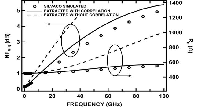
Fig. 4. Simulated and extracted  $NF_{MIN}$  and  $R_n$  with and without correlation at minimum noise bias. The emitter area is  $0.2 \times 1 \mu\text{m}^2$ .
