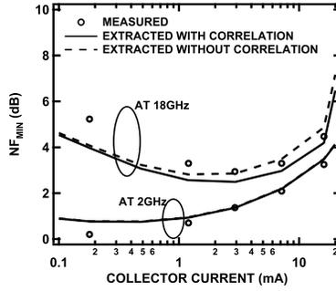
Fig. 8. Measured and modeled  $NF_{MIN}$  at 2 and 18 GHz vs.  $I_C$  (with pad parasitics).
