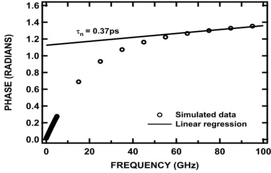
Fig. 3. Extracting noise transit time  $\tau_n$  from the high frequency transconductance of the simulated SiGe HBT.
