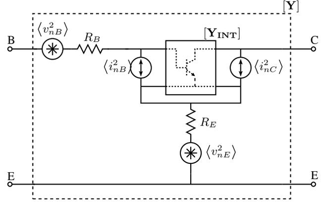
Fig. 1. SiGe HBT noise equivalent circuit defining the intrinsic and extrinsic  $y$ -parameters
