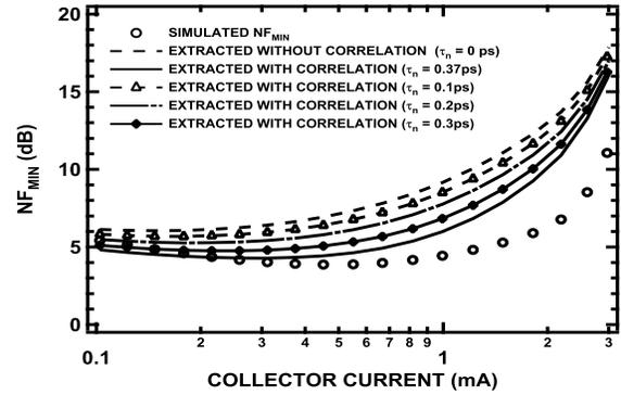
Fig. 6. Simulated and extracted  $NF_{MIN}$  at 65 GHz for different values of  $\tau_n$ . The emitter area is  $0.2 \times 1 \mu\text{m}^2$ .
