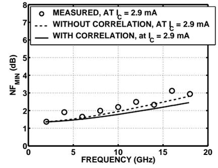
Fig. 9. Measured and modeled  $NF_{MIN}$  at minimum noise bias (with pad parasitics).
