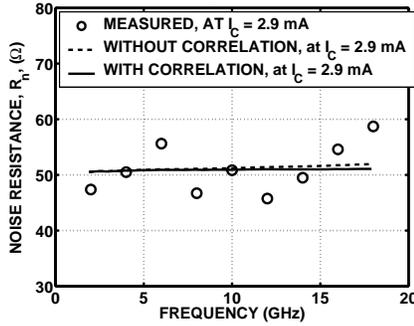
Fig. 10. Measured and modeled  $R_n$  at minimum noise bias (with pad parasitics).
