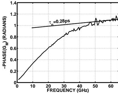
Fig. 7. Measured phase of  $g_m(\omega)$  at  $V_{CE} = 1.5 V$ .
