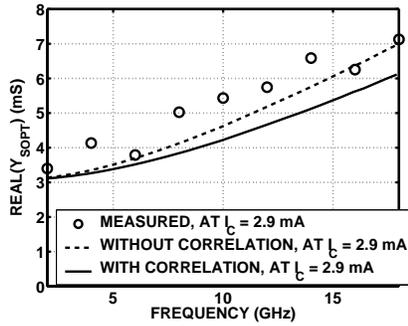
Fig. 11. Measured and modeled  $\Re(Y_{SOPT})$  at minimum noise bias (with pad parasitics).
