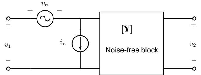
Fig. 2. Chain matrix representation of a linear noisy two-port network.
