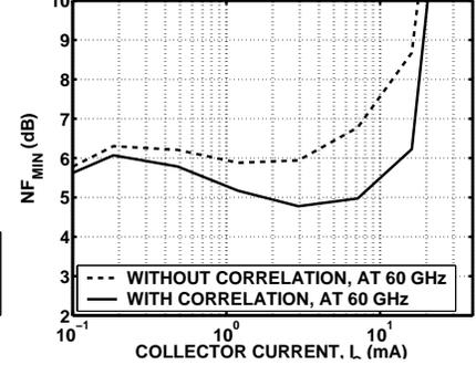
Fig. 12.  $NF_{MIN}$  vs.  $I_C$  at 60 GHz as extracted from  $y$ -parameters after de-embedding pad parasitics.
