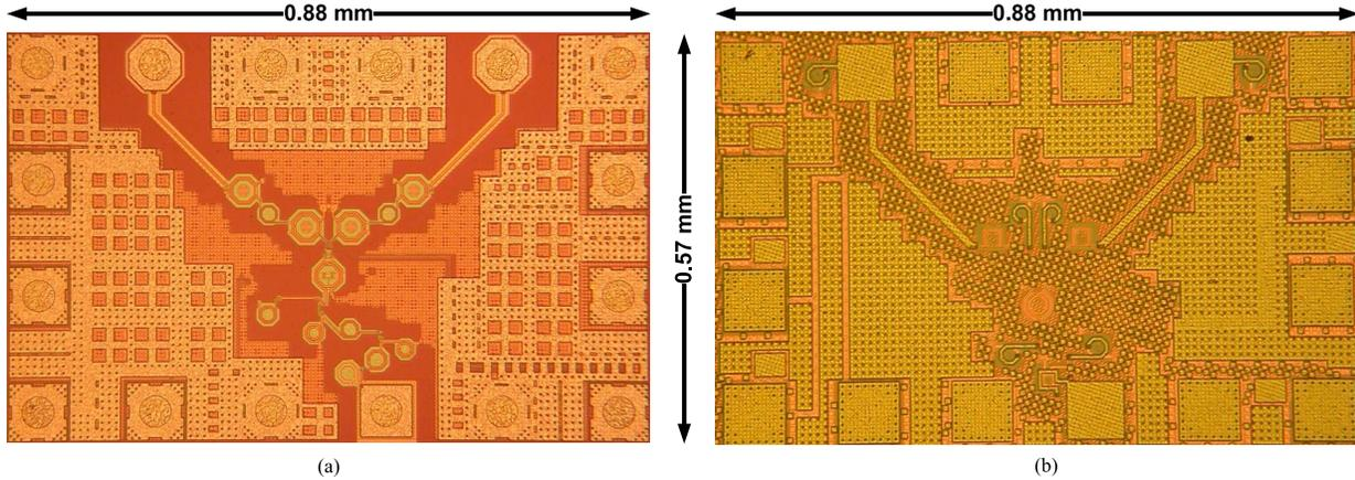
Fig. 16. Chip microphotograph of the mm-wave tag in (a) 55-nm SiGe BiCMOS and (b) 45-nm SOI CMOS technologies. Both chips have a size of  $0.57 \times 0.88 \text{ mm}^2$ .
