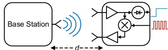
Fig. 1. FMCW radar system consisting of base station and active tag.
