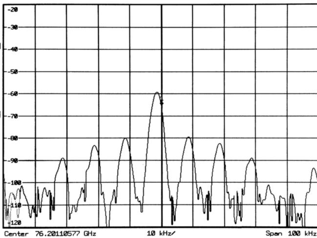
Fig. 28. Measured spectra, in dB, of a received 76.2-GHz carrier AM-modulated by a 10-kHz sinusoid applied at the gain-control pads of the packaged SiGe tag placed 5 m away from the base station.
