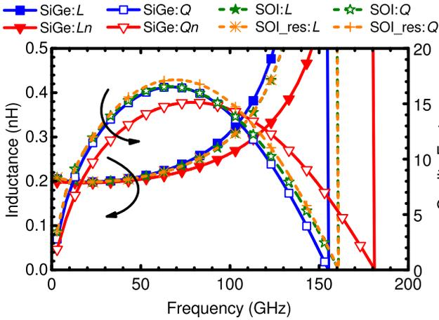
Fig. 7. EM simulation of effective inductance  $L$  and quality factor  $Q$  of the same inductor realized in the 55-nm SiGe BiCMOS BEOL (SiGe) and 45-nm SOI CMOS BEOL with  $10\text{-}\Omega\times\text{cm}$  (SOI) and  $1000\text{-}\Omega\times\text{cm}$  (SOI<sub>res</sub>) silicon substrates.  $L$  and  $Q$  describe the inductor with  $30\text{-}\mu\text{m}$  diameter in both BEOLs, whereas  $L_n$  and  $Q_n$  describe the  $26\text{-}\mu\text{m}$ -diameter inductor in the SiGe BEOL.
