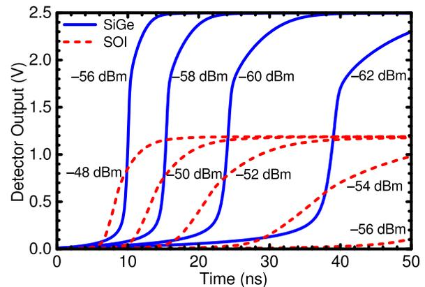
Fig. 14. Simulated SiGe and SOI tags wake-up time as a function of input signal power at 80 GHz.
