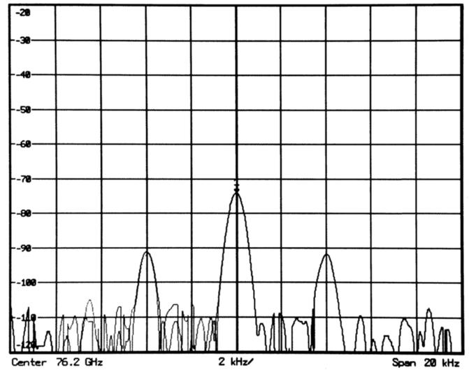
Fig. 27. Measured spectra, in dB, of a received 76.2-GHz carrier BPSK-modulated by a 4-kHz sinusoid applied at BPSK pad of the packaged SiGe tag placed 5 m away from the base station.
