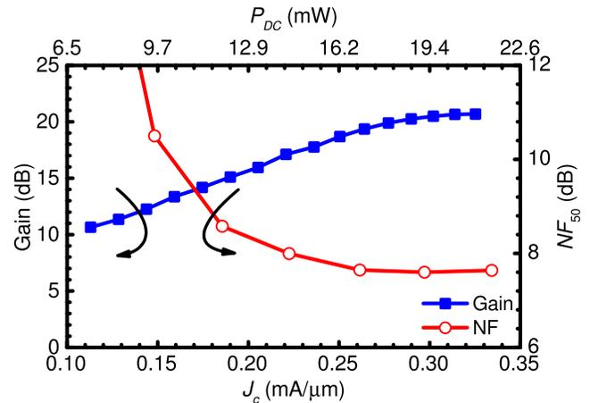
Fig. 21. Measured gain from the input to one output and  $NF_{50}$  versus current density for the SOI tag at 78 GHz.
