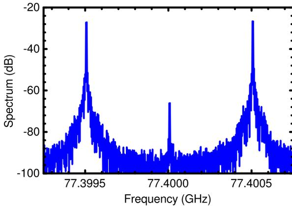
Fig. 24. Spectra of a 77.4-GHz carrier BPSK-modulated with a 500-kHz sinusoid for SOI tag.
