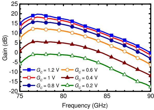
Fig. 23. Measured tag gain from the input to one output as a function of the gain control voltage and frequency SOI tag.
