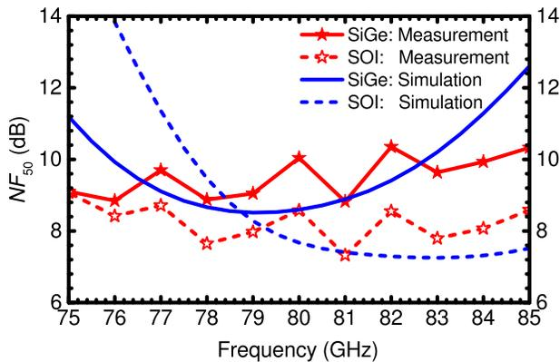
Fig. 19. Measured and simulated tag  $NF_{50}$  in the W-band. Solid and dash lines correspond to SiGe and SOI tags, respectively.
