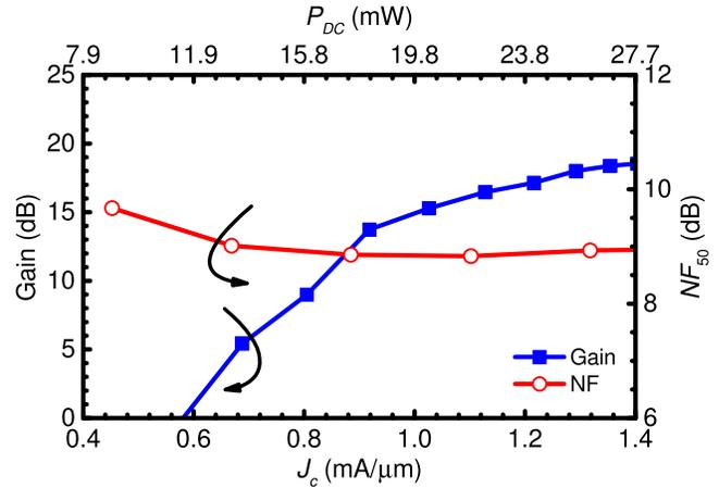
Fig. 20. Measured gain from the input to one output and  $NF_{50}$  versus current density for the SiGe tag at 79 GHz.
