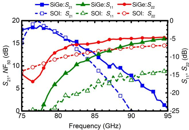
Fig. 18. Measured tag S-parameters in the W-band. Solid and dash lines correspond to SiGe and SOI tags, respectively.
