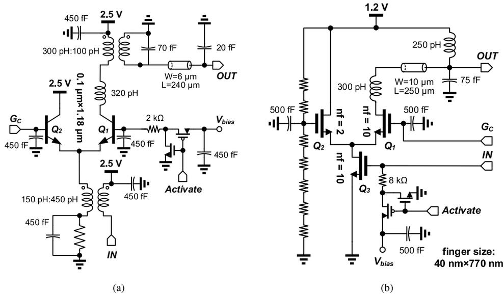
Fig. 15. Schematic of the VGA block implemented in (a) 55-nm SiGe BiCMOS and (b) 45-nm SOI CMOS technologies.
