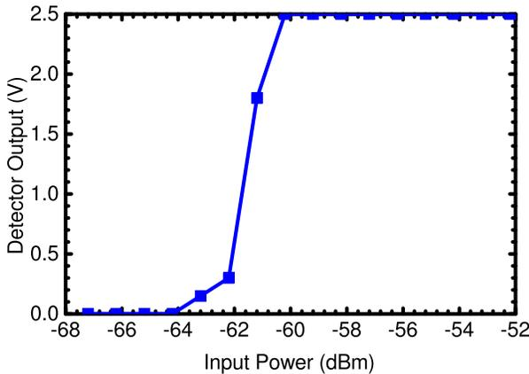
Fig. 25. Measured SiGe tag detector output voltage versus input power.
