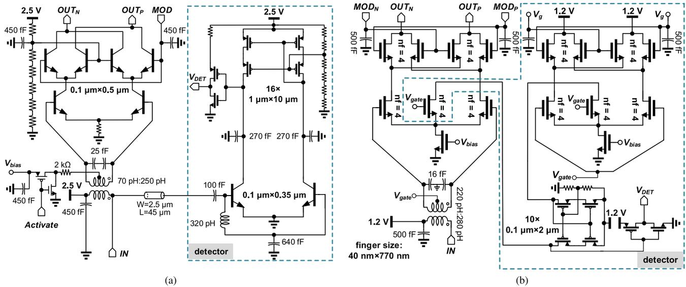
Fig. 12. Schematic of the modulator and detector block implemented in (a) 55-nm SiGe BiCMOS and (b) 45-nm SOI CMOS technologies.
