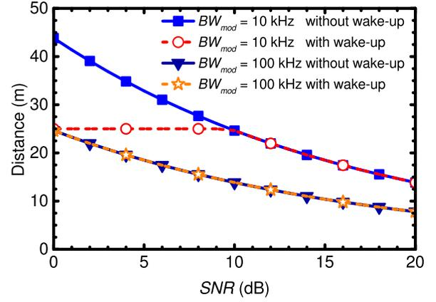
Fig. 2. Link distance versus base station receiver SNR for two different values of the tag modulation bandwidth, with and without wake-up functionality.
