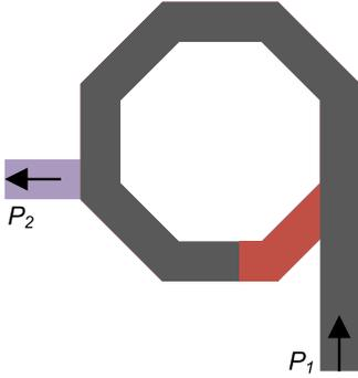
Fig. 6. Three-turn inductor layout realized in the aluminum and top two copper layers.
