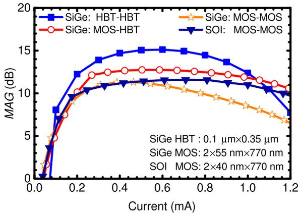
Fig. 3. Simulated MAG at 80 GHz as a function of current for minimum-size cascode stages in 55-nm SiGe BiCMOS and 45-nm SOI CMOS technologies.
