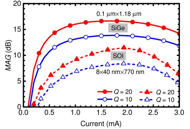
Fig. 8. Simulated MAG at  $80\text{ GHz}$  versus current of HBT-HBT cascode in 55-nm SiGe BiCMOS and MOS-MOS cascode in 45-nm SOI CMOS technologies for output matching quality factors of 10 and 20.
