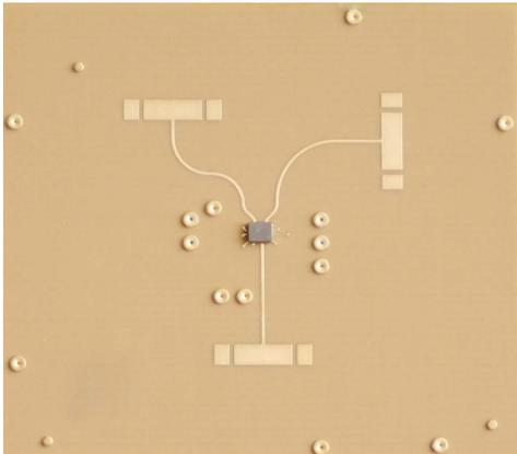
Fig. 17. Tag chip flip-chip mounted on a  $23 \times 20 \text{ mm}^2$  mini-PCB with two transmit and one receive antennas.
