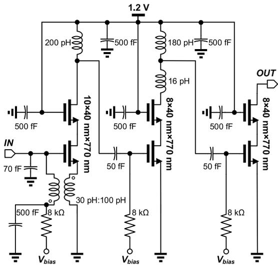
Fig. 11. Schematic of the LNA block implemented in 45-nm SOI CMOS technology.
