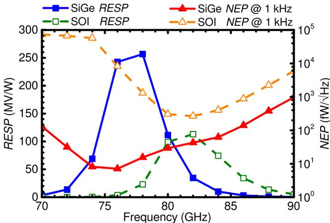
Fig. 13. Simulated *RESP* and *NEP* versus frequency for SiGe and SOI detectors.
