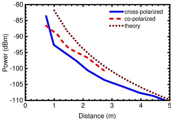
Fig. 29. Received copolar and cross-polar sideband power versus distance in the base station-tag measurement setup. The dotted line shows the theoretical expected power level.
