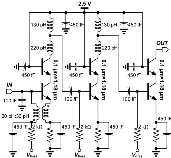
Fig. 10. Schematic of the LNA block implemented in 55-nm SiGe BiCMOS technology.
