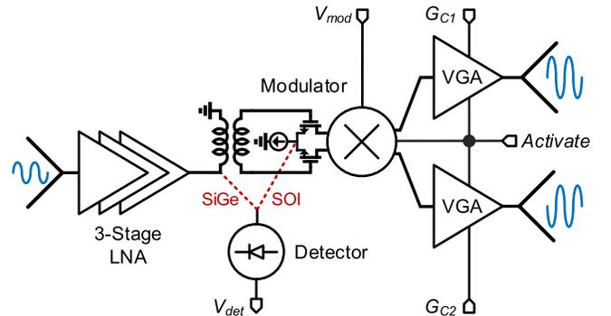
Fig. 9. Block diagram of the mm-wave tag. The detector block connection in the SiGe and SOI implementation is shown with the dashed line.
