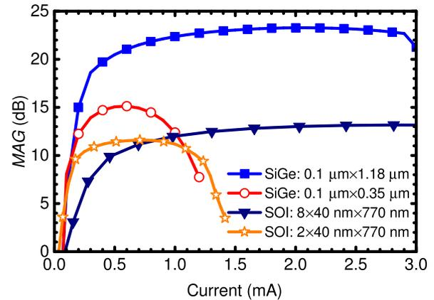
Fig. 4. Simulated MAG for HBT-HBT and MOS-MOS cascodes of two different sizes in 55-nm SiGe BiCMOS and 45-nm SOI CMOS technologies, respectively.
