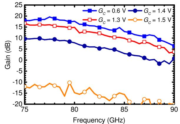
Fig. 22. Measured tag gain from the input to one output as a function of the gain control voltage and frequency in SiGe tag.
